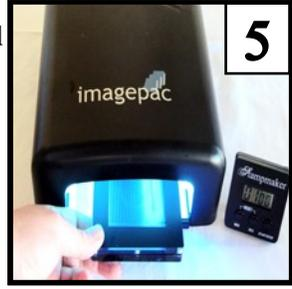
**5** With the negative facing up, insert the clamp fully into the Stampmaker for 1 minute. **Use a separate timer.**
