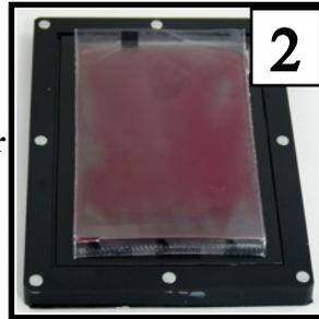
**2** Place the emboss imagepac on top of the BLACK spacer. Ensure the word 'imagepac' is face down.
