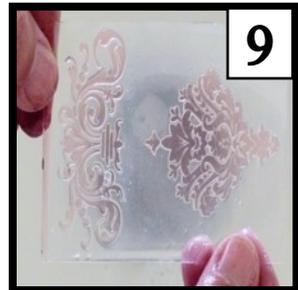
**9** Take care to ensure you have washed it fully to remove any traces of liquid polymer before the second exposure.
