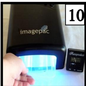
**10** Put 1/4" of cold water in the exposure tray and place the emboss in. Then put the tray into the Stampmaker for another 2 minutes to harden the polymer.
