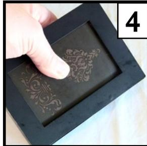
**4** Place the lid of the clamp on and squeeze the center of the clamp firmly for 10 seconds to spread the polymer evenly inside the imagepac.
