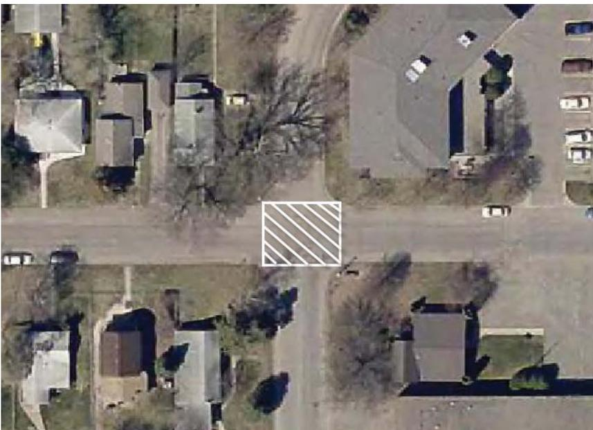
Given the current budget constraints of the city and the modest volume of traffic – both pedestrian and automobile – in this corridor, the interim approach of crosshatching is a prudent step to take to address the current safety problem.
