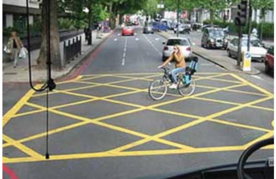
Crosshatching is an inexpensive, short term fix. Changing the dimensions and function of 5th Avenue, adding sidewalks to D Street and tightening the intersection with concrete bump outs are longer term solutions, but they have a much greater expense.
