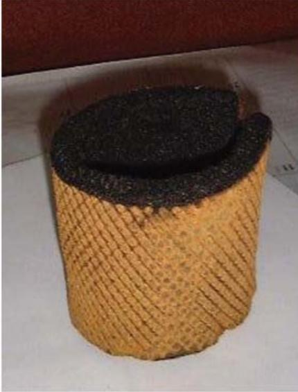
**Figure 2: Loaded cathode**
