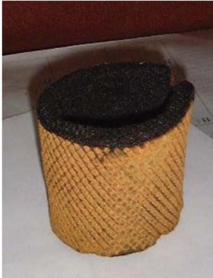
**Figure 2: Loaded cathode**
