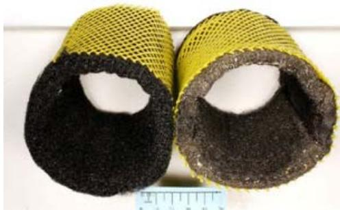
**Figure 3: Comparison photograph of new cathode (left) and PGM-loaded cathode (right)**
