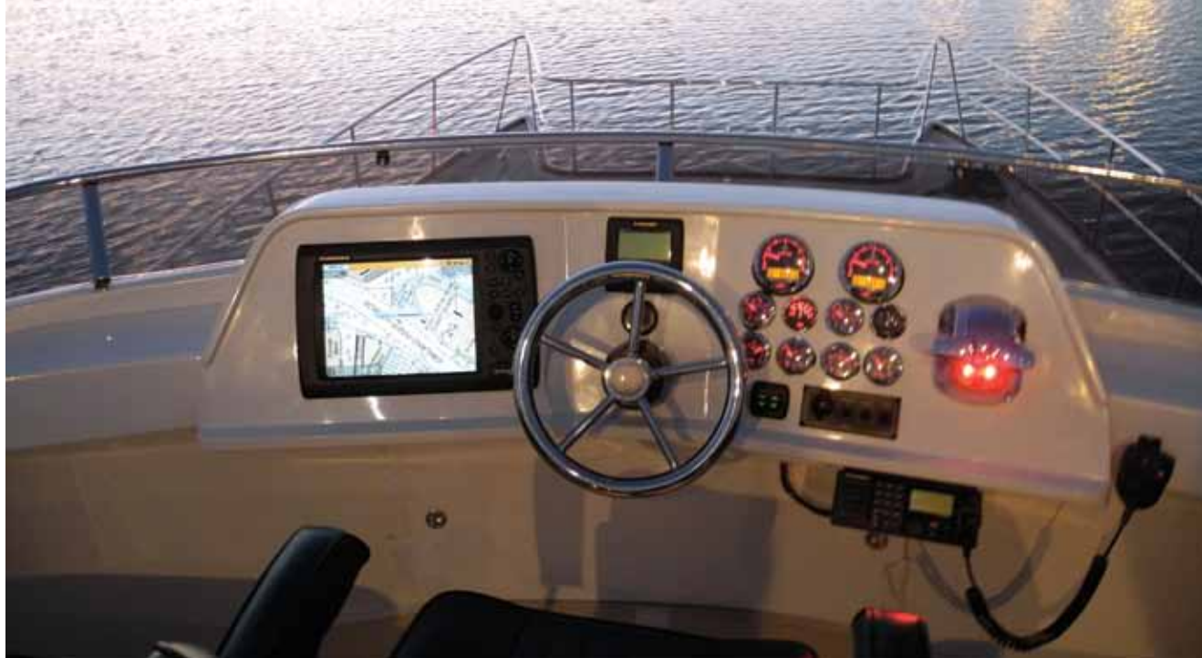
The centerline bridge helm has excellent views of all four corners of the boat, plus a complete set of engine performance gauges mirroring those in the pilothouse, as well as a remote multifunction display.
