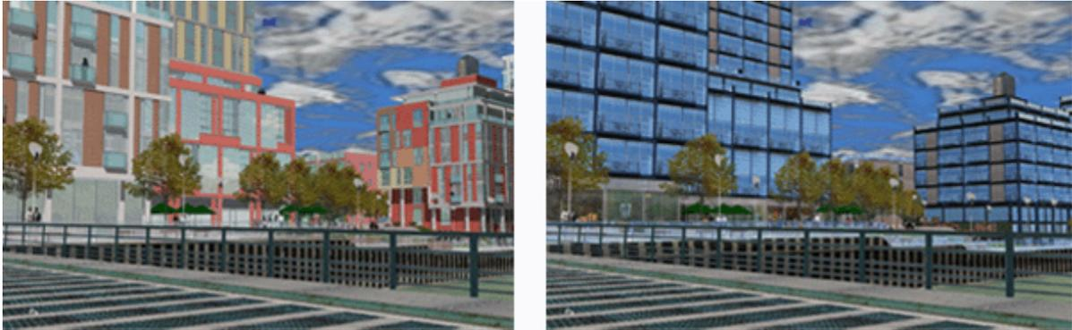
*Final Design Phase: Textured 3D models of two alternative facades in an immersive 3D environment. This level of detail would be used during the final stages of the approval process and the public hearing. (Image credit: Michael Kwartler & Environmental Simulation Center, Ltd.)*
