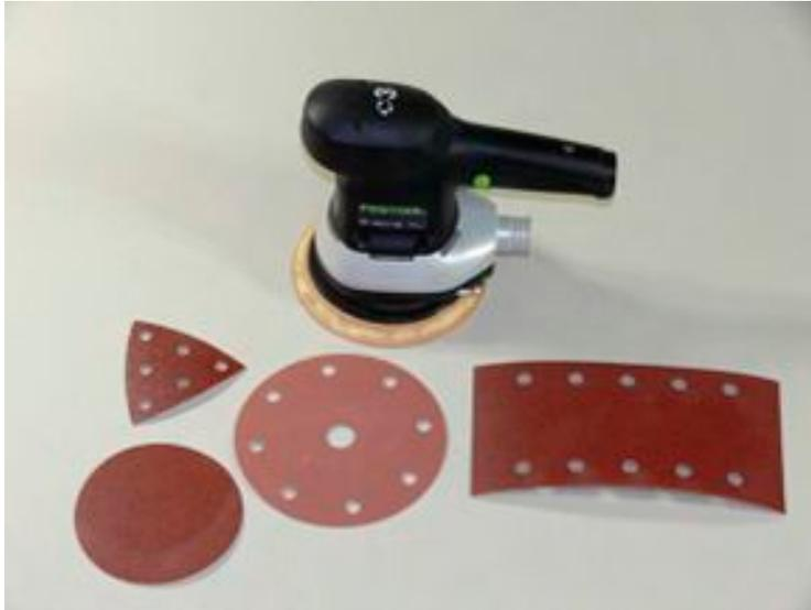
Random orbit machines *rotate a pivot point while allowing the attached but not mechanically driven pad to move*
