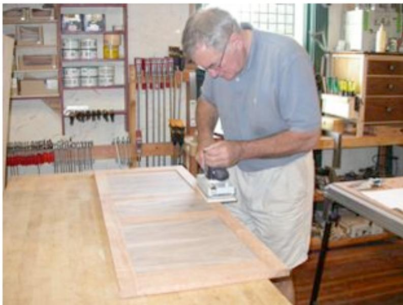
As pictured here you can see how the large flat surface is ideal for rail, style and panel components where a tip of the sander could well leave an undesirable depression along an edge.
