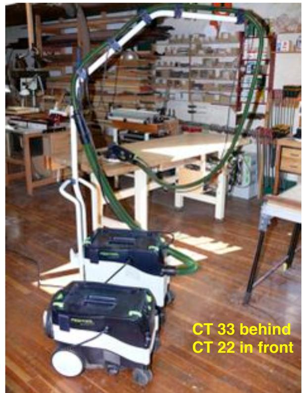
gets taller. A CT 22 is shown in front of a CT 33 in the photo on the previous page. Notice how the white lower section is taller on the CT 33 than on the CT 22. They draw 134 CFM and pull an impressive 90" of static water lift (23000Pa) while generating only a 72dB noise level.
