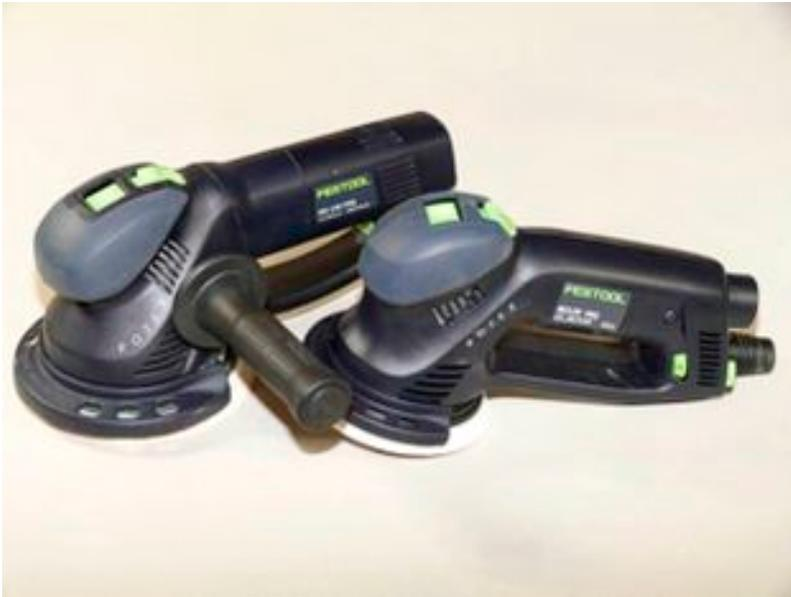
action. The green switch on the top makes the mode change. In one mode they act just like the ETS random orbit units. Switch modes on the RO 150 or the RO 125 and things get very different. The second mode on both machines is a hybrid between the gear driven pure rotary motion of the RAS 115 and the pure random orbit motion of the ETS units.
