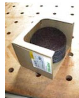
aluminum oxide and silicon carbide particles embedded in a synthetic fiber mat allowing it to easily follow surface contours and to reach into surface imperfections. It does a great job of cleaning most anything and in coarser grits can be quite aggressive.
