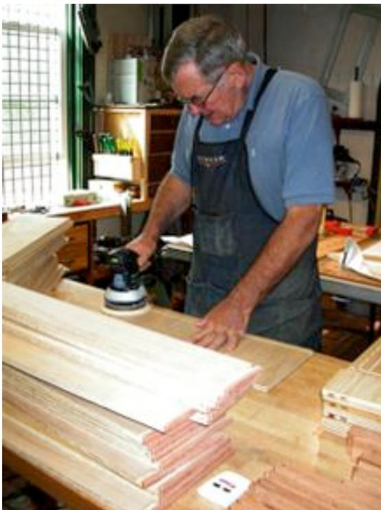
*in a random motion.* This produces very fine finishes with little or no scratching so long as you keep the pad flat on the work surface. Tip the pad to get more aggressive stock removal and scratches are sure to be the result.
