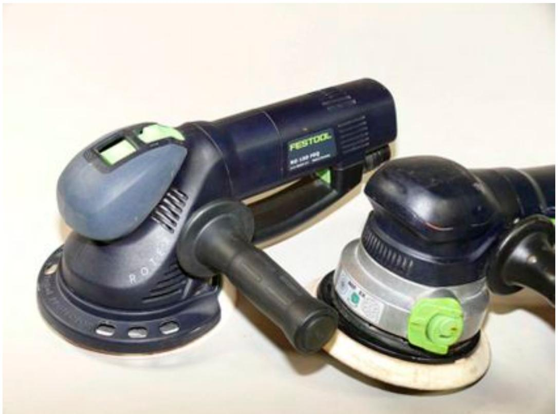
150mm (6") pad unit or the 125mm (5") unit (both shown here for size comparison), feature a switch selectable sanding
