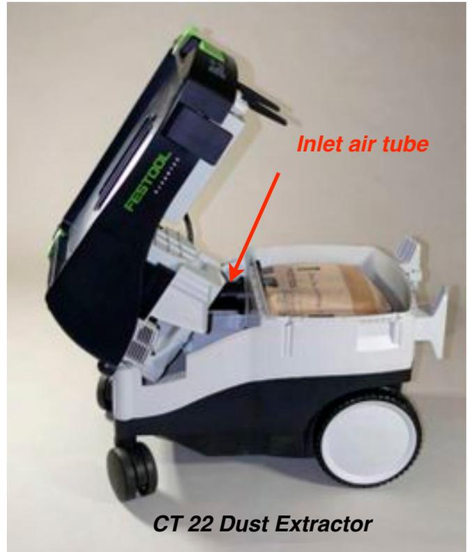
The CT 22 and larger units are different. First, the top hinges open rather than lifting off. The disposable bags fit into a chamber tightly connecting to the incoming air hose tube shown in the photos above and to the left.
