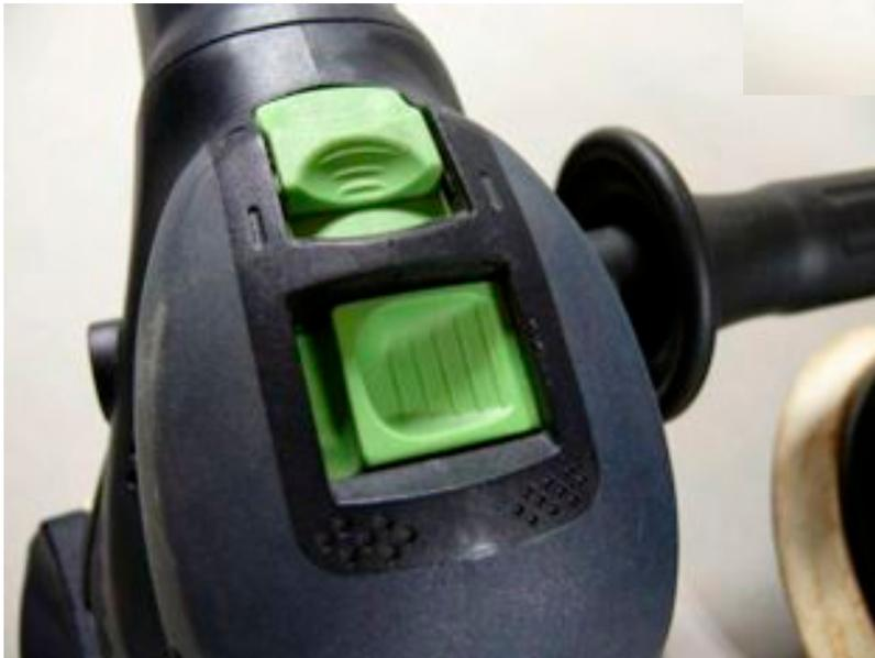
new version the same change is accomplished by simply moving the green rectangular button on the front top of the unit. Faster and far handier. The other green button shown is the on-off switch positioned to be on top right where your
