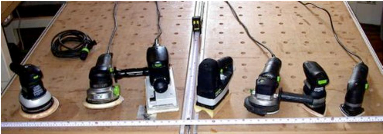
There are basically three different ways the abrasive can be moved by a machine sander: **linearly in a fore-aft motion, in a circle in a rotary motion, or back and forth in an arc.** Festool uses the first two motions but not the arc motion.
