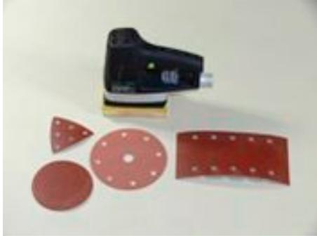
any other means. Sanders which move the pad in any direction other than purely linearly will create a flat spot on any linear curved surface like a stair handrail. With the LS sander you can easily do rebates (rabbets), edges, or profiles that otherwise would require laborious hand sanding.
