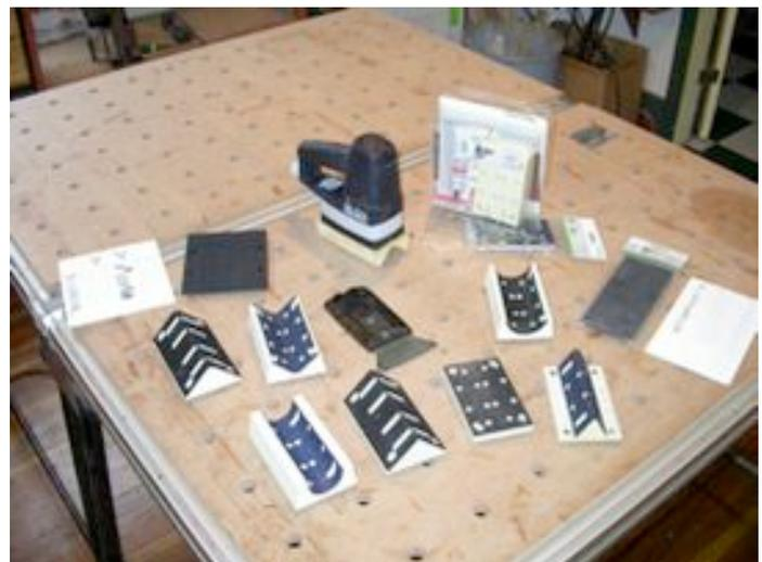
center of this photo) is offered as an accessory. Since the motion of the LS 130 is purely fore and aft you can use this to scrape off wallpaper, carpet, and other glued on materials far more easily than you could do by hand.
