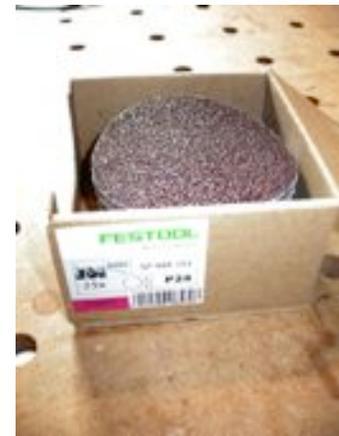
The heavy cloth type backing can take more heat and abuse than the paper backed materials used on Brilliant, Cristal and Rubin. While it can take more heat, be careful as it is very aggressive and can remove a lot of stock very quickly. In the process a lot of heat can be generated. Use a light touch and the results are very impressive.
