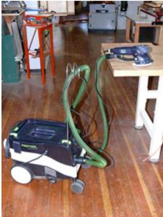
with all of the Festool sanders and cutting tools. Combined with the 9 hole vent pattern in the round pad sanders, and the variety of hole patterns in the other sanders, this potent team keeps the air around the sanding area much cleaner and safer for the person operating the sander.
