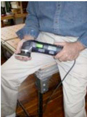
you constantly move the machine, the same sanding grit passes the surface of the work piece at the same location repeatedly leaving often hard to remove deep scratches. The DX sander does not do this
