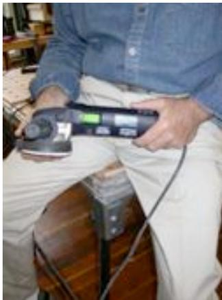
The RAS sander is also very handy for removing paints, rust or surface contaminants as long as you keep in mind just how much heat doing so can generate. You don't want to burn the work piece nor do you want to burn and ruin the pad.
