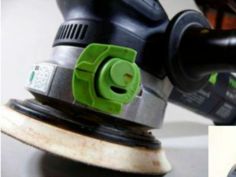
On the previous version changing from rotary to random orbit mode required lifting the lock and twisting a shaft, the green mechanism shown in this photo. Simple enough but a bit fussy. On the
