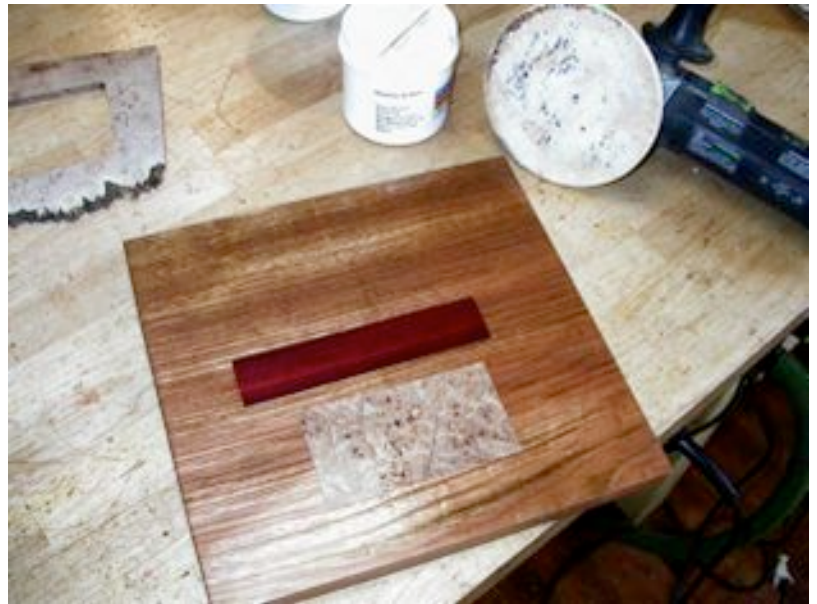
Open field inlay in sample piece after being polished with the Festool RO150. The field is Brazilian cherry. The dark red inlay is South African blood wood. The lighter colored inlay is Oregon Big Leaf maple burl that was cut from the piece above.
