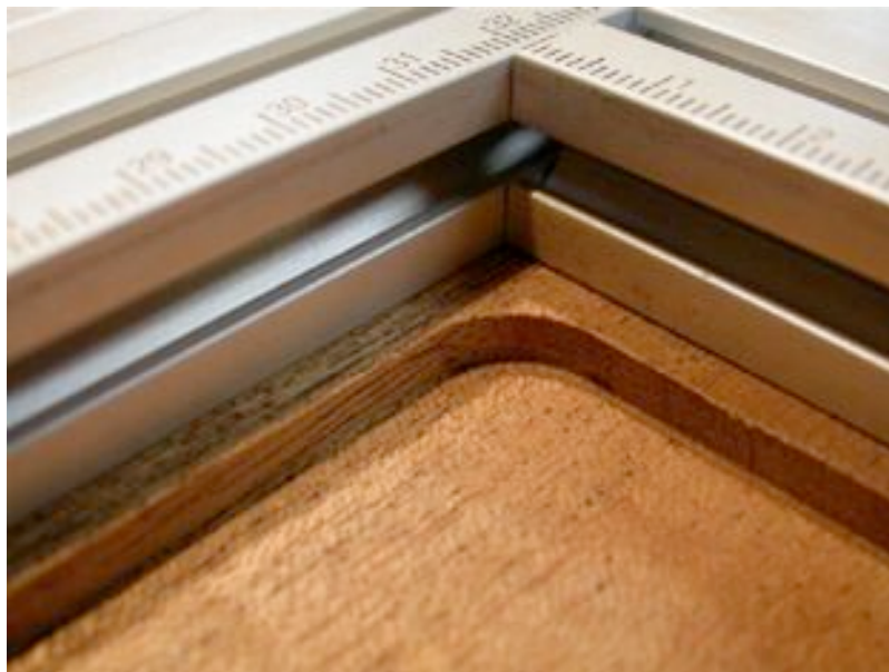
Open field inlay in sample piece after being polished with the Festool RO150. The field is Brazilian cherry. The dark red inlay is South African blood wood. The lighter colored inlay is Oregon Big Leaf maple burl that was cut from the piece above.
