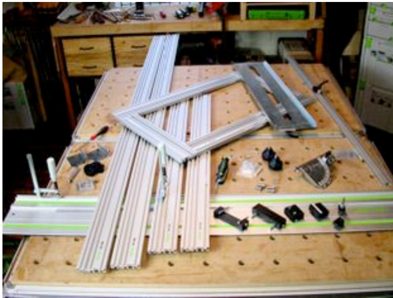
MFS system shown here with shop made accessories as well as Festool supplied components.
