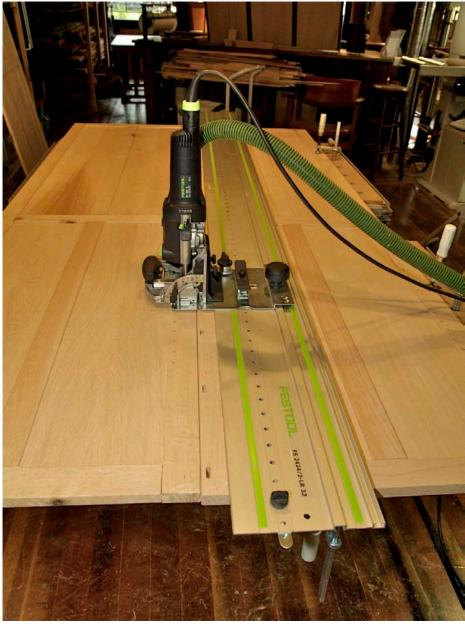
method for mounting the Domino machine onto the indexing sled of this jig instead of the router with which the jig is normally used.
