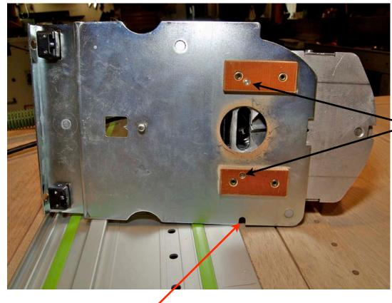
19mm from each edge of the center hole in the sled as shown in the photo below. You want to be as precise with these locations as you can to properly register the Domino relative to the sled and make sure it sits flat on the top surface of the sled with both pins fully seated in the new holes you drill through the base of the sled.
