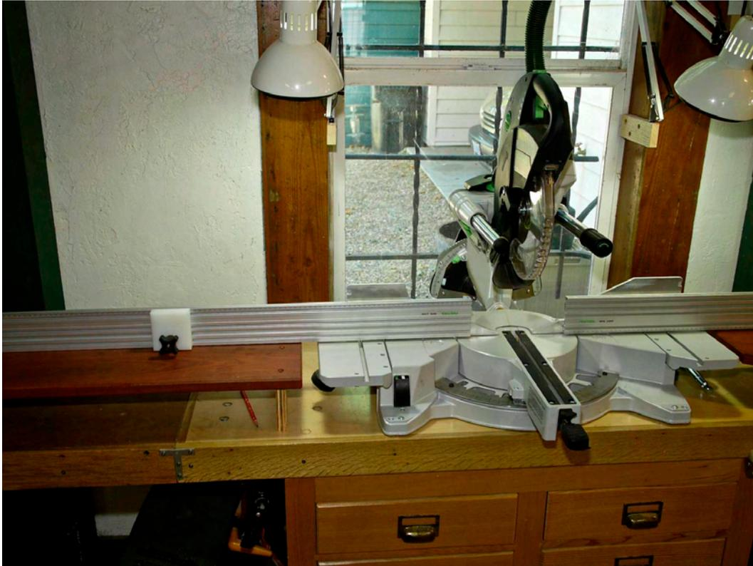
Most who use the Festool Kapex compound sliding miter saw will want to add some form of side stops to allow fast and easy repeat cutting of parts the same length. Stops are all the more useful if there is a measurement scale calibrated to the saw blade that allows you to set the desired length of cut without measuring and marking.
