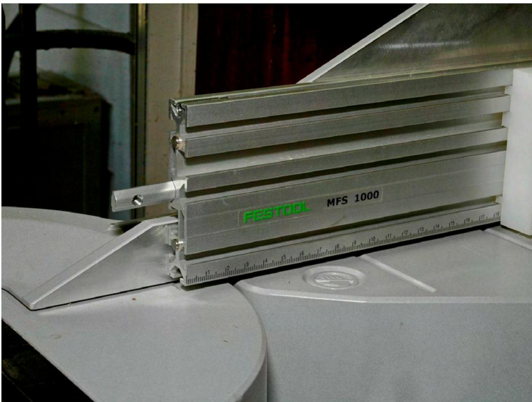
removable wing fences on the Kapex that align with this middle “V” track while the MFS profile is about 5mm above the Kapex table surface.
