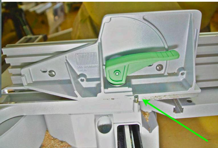
Here is what it looks like with the holes drilled in the wing fence, the wing fence in place on the Kapex and the two MFS joining units (red arrow) screwed partially onto the 10-32 x 1/2" machine screws.
