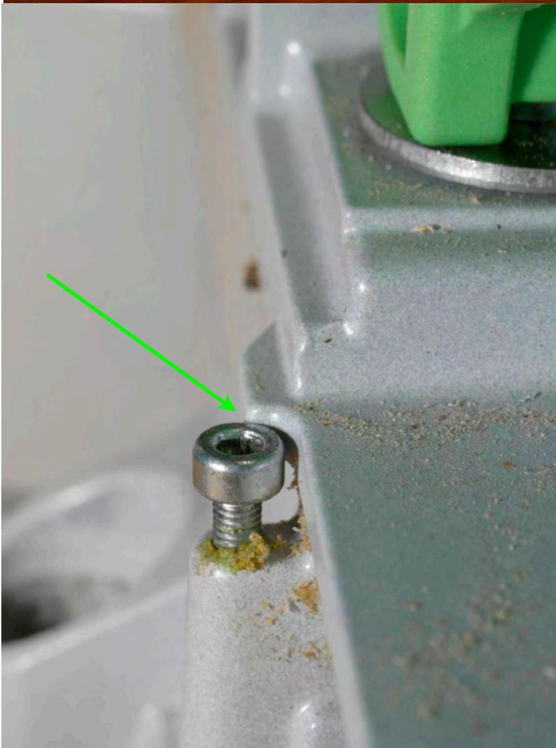
Note in the photo left that the Kapex has a built in wing fence stop screw (green arrow) that will register the wing fence in the same place time after time even when you remove and replace the fence. To remove the fence, lift the green lock lever, screw down the stop screw and slide the fence off the Kapex. To replace the fence, slide it in place, raise the stop screw, slide the wing fence over to hit the stop screw and press down the green lock lever.
