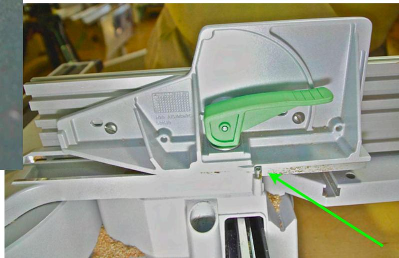
Here is what it looks like with the holes drilled in the wing fence, the wing fence in place on the Kapex and the two MFS joining units (red arrow) screwed partially onto the 10-32 x 1/2" machine screws.
