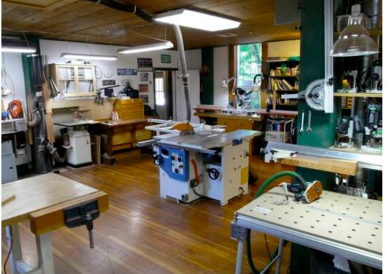
The upper photo shows the Kapex work center looking past the band saw center (this one a 24" band saw) and the four Festool MFT assembly tables.
