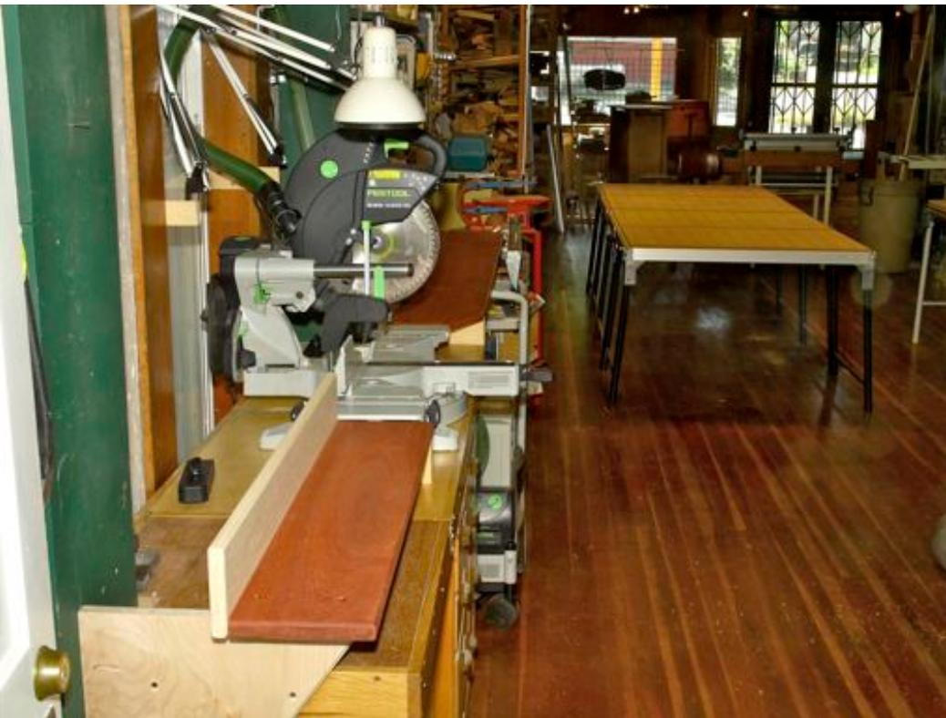
You can see just how closely the Kapex hugs the wall and it projects out into the room no further than the dust collector, or the orange Heigner scroll saw or the wood storage racks beyond it. It simply tucks in out of the way very unlike all the other CMSs I tried and removed from the studio as they simply took up too much space.
