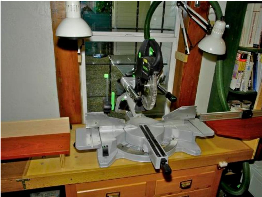
Note also that I set the in-feed and out-feed tables and fences so they are far enough away from the available Kapex add on wings that the wings can be removed or placed without moving the saw or the tables/fences.
