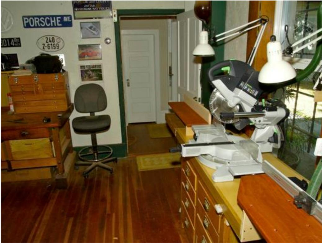
Here are shots of the Kapex work center looking both directions. The top photo is from the out-feed side looking across the in-feed table and fence that allows long work pieces to project into the open door way.
