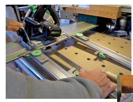
the fast fix lever and lock the blade down into the blade change position. Set the rear stop "V" mark exactly on a measure (in this case 400mm). The distance from the point of the "V" mark to the edge of the rule is about 1mm, so I like to use a magnifying glass to make sure the stop is set correctly before I calibrate or set up for a critical cut.
