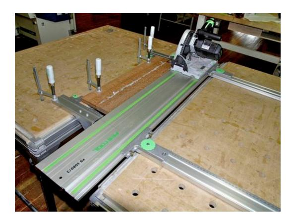
Story sticks made to hold the guide rail a known distance from the edge at both ends really make it fast and easy to make perfect parallel cuts time after time. That is what Festool has done with its new Parallel Guide system which we will cover in this short tutorial. While it sounds simple, and it is, the new Parallel Guides also make an excellent squaring cut guide as well turning the guide rail and plunge saw into a fast and efficient substitute for a table saw for most cutting operations.
