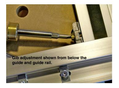
The distance between the brass gib screws (red arrow) is 110mm, almost twice the purchase distance of a steel rule mounted in a Starrett combination square head. The cast metal "T" bracket is positioned on the extruded aluminum guide by a molded ridge that rides in a slot in the extrusion (green arrow).
