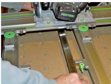
Since you are calibrating the two parallel guides to the guide rail, saw and blade all at the same time, be sure to recheck calibration any time you change blades. It actually takes longer to describe than to
