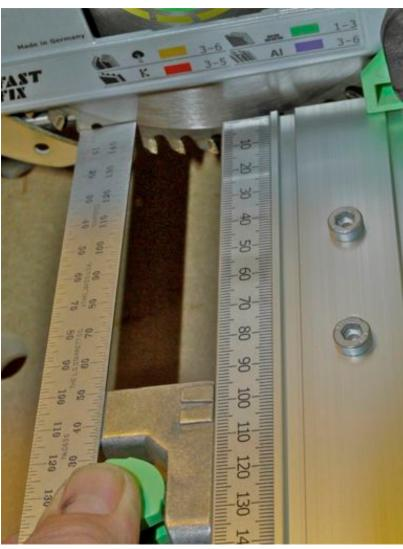
In these photos I am calibrating the stop to the front scale. Notice I have the "V" cast into the stop aligned with 100mm on the scale yet my rule that is touching a tooth on the blade (photo above) shows the distance to the stop as being slightly less than 100mm.
