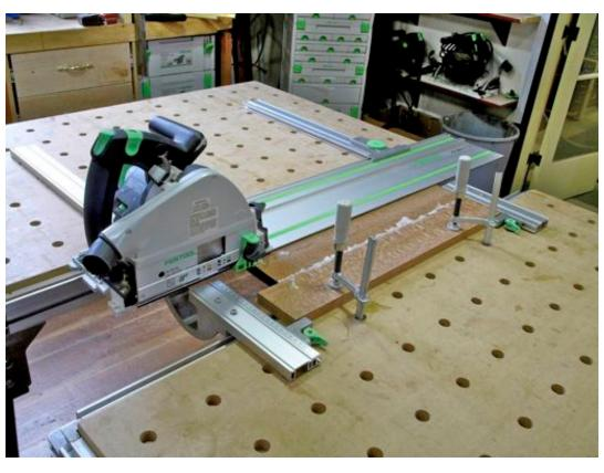
other edge was a break off so had an uneven, waney edge. I wanted the shelf to wind up 160mm wide by 540mm long, a size difficult to cut with the guide rail mounted to the MFT as it is narrower than the guide rail itself.
