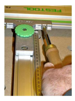
The parallel guide simply slides onto the rear "T" track of the guide rail with a locking tab (accessed from below)
