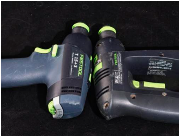
15+3 compared to the older TDK 15.6. To overcome the natural perspective distortion I placed the T 15+3 both in front of and behind the TDK 15.6 in the comparison photos. Note that the back edges of the motor housings are aligned to show just how much shorter the 15+3 really is. Slick!
