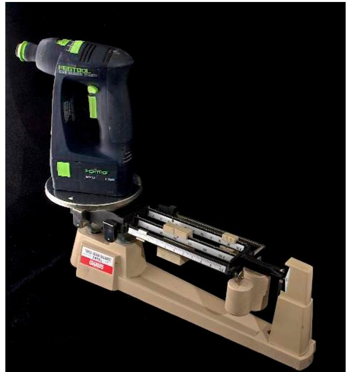
Here and on the previous page are photos of the two extremes, a NiMH C-12 and a Li-ion T 15 + 3. They are surprisingly similar in terms of size, weight, and balance even though they employ completely different form factors and different battery technology.
