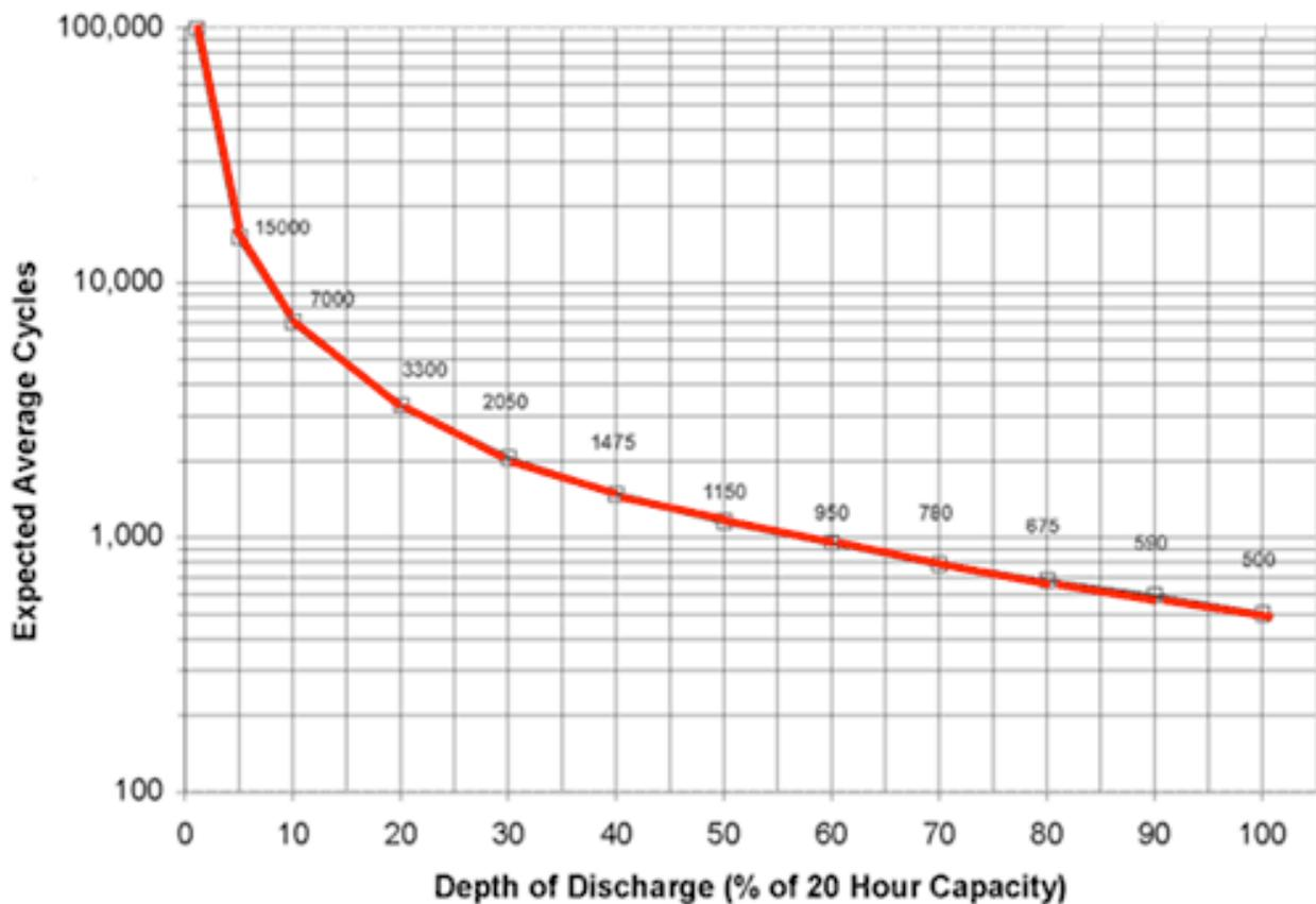
On the vertical axis is the total number of discharge/recharge cycles the battery can stand before it fails. On the horizontal axis is the depth to which the battery is
