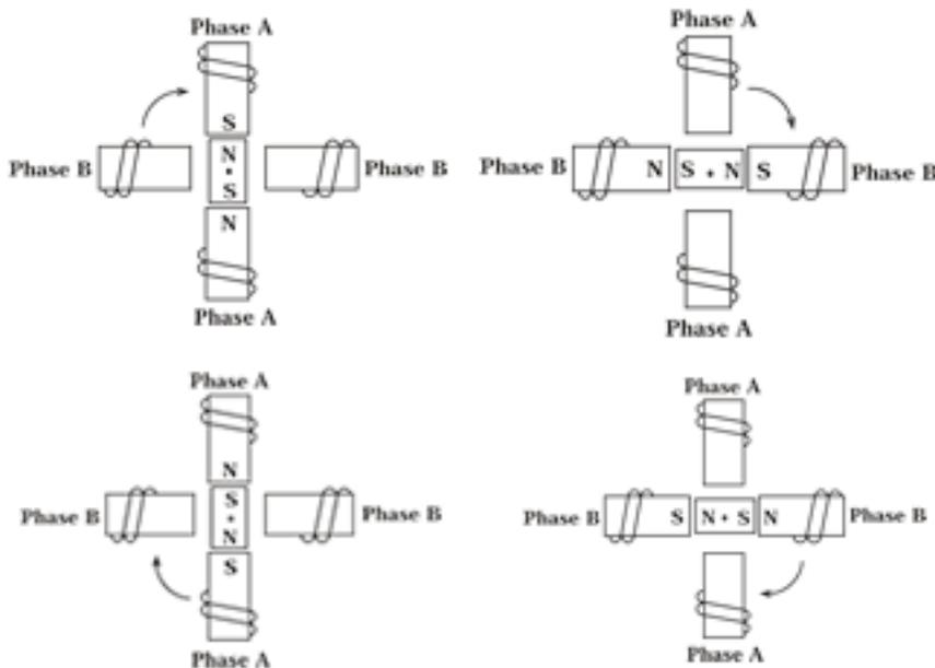
If you were to energize two of the electromagnets at the same time, the north and south poles on the permanent magnet would experience a greater magnetic attractive force creating more turning force or torque, about 40% more. But, since two, rather than one, of the electromagnets is energized at the same time the motor will consume twice the number of electrons. Each rotational step of the motor shaft would be at 45 degrees to the poles of the stationary magnets as shown right.
