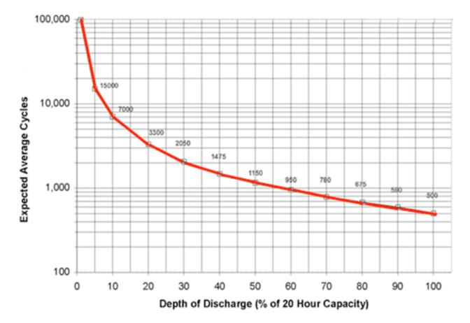
On the vertical axis is the total number of discharge/recharge cycles the battery can stand before it fails. On the horizontal axis is the depth to which the battery is
