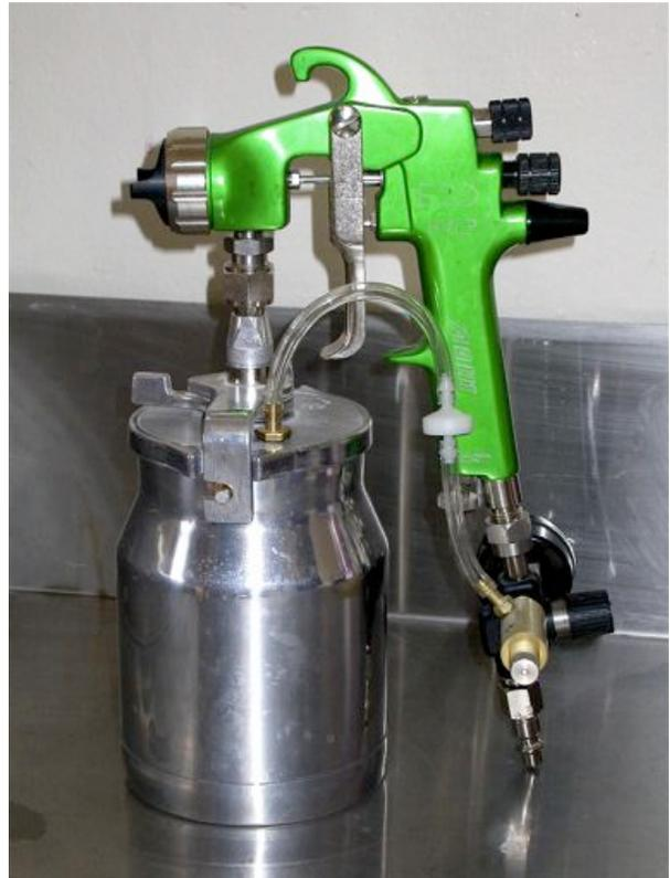
I had a hard time warming up to this gun. I found the add on pot pressure contraption awkward even though it does allow individual control over pressure in the pot. I suppose there is an advantage to being able to control the amount of pot pressure which you can do with this gun but not with either of the other two PP guns, but I was not able to really explore this in these tests.
