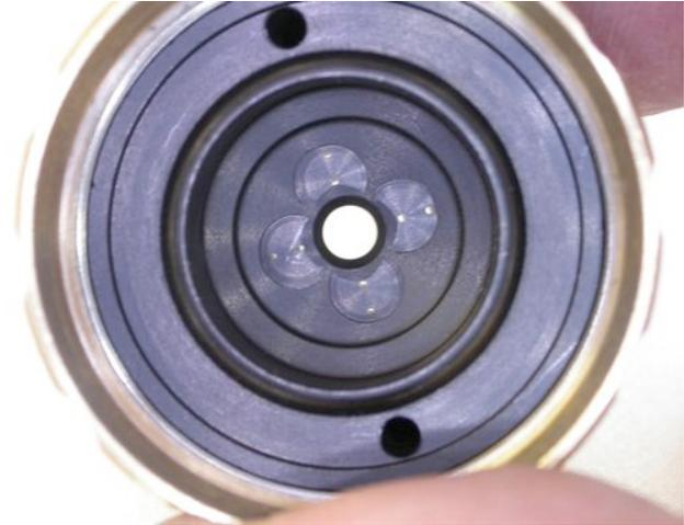
Look again at the photo to the left and see how the outer holes provide the fan control air and the inner holes provide the atomization air. No accidental engineering here.
