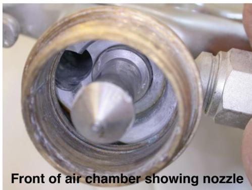
Front of air chamber showing nozzle
