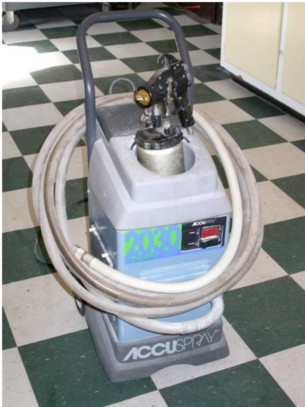
**Accuspray three stage turbine and non-bleeder gun**
