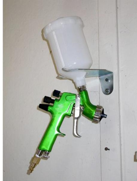
**Asturo gravity feed HVLP gun (above) and High Transfer Efficiency gun (below)**
