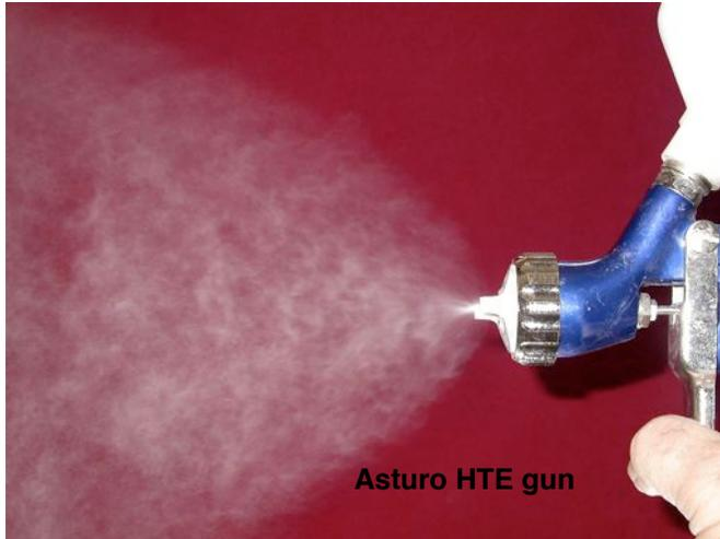
The round, soft and full fan pattern produced by the Asturo HTE conversion gun produced outstanding finish results with all the different finish materials. The Asturo HVLP gun fan pattern, shown below is sharper edged and somewhat harder, but also produced very nice results.
