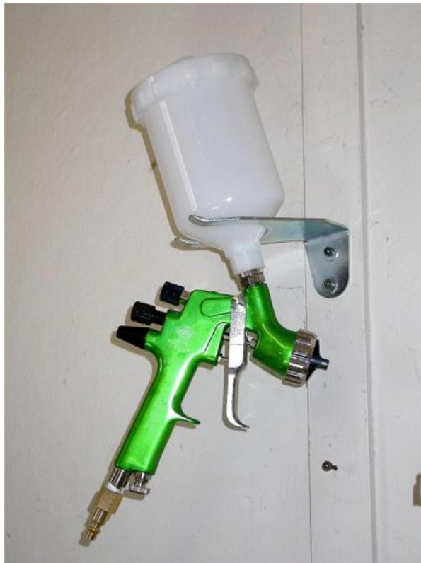
The conversion guns did not appear to use a great deal of air. My compressor is only a standard four HP 220 volt cast iron single stage unit with a 20 gallon horizontal tank. It cycled on and off in use a bit but nothing excessive. I think I could use these conversion guns all day long and not over tax this small compressor.
