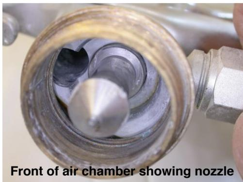
Front of air chamber showing nozzle
