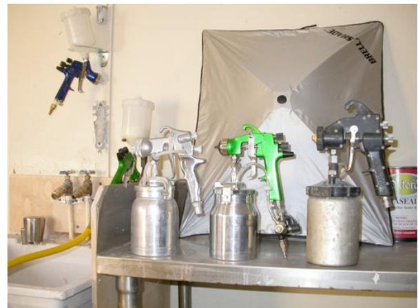
**This photo shows (left to right) the Apollo turbine pressure pot gun, Asturo HVLP conversion PP gun and Accuspray turbine PP gun.**
