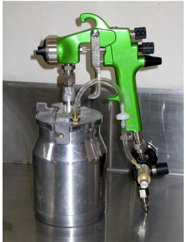
**Pressure pot gun shown above and a gravity feed gun is shown at left. Both are Asturo HVLP conversion guns.**
