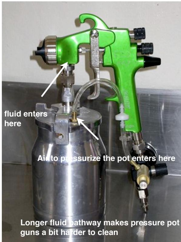
The pressure pot guns are also easy to clean, just not as easy as the gravity feed guns. From the picture above you can see that the fluid is contained in the cup below the gun and the cup is pressurized by the incoming air stream. In the case of this Asturo gun the pressure tube leads from a pressure controller screwed to the inlet port on the end of the handle.
