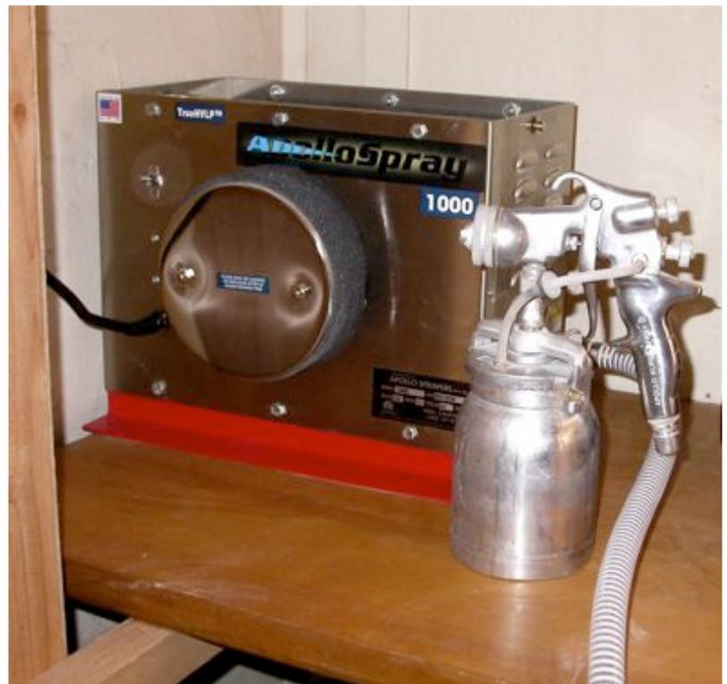
The trade off is, ***this sucker is loud.*** Where a compressor emits a low frequency pounding sound, this Apollo turbine emits a high frequency whine that would be hard to live with if it was in the same room where you were spraying.
