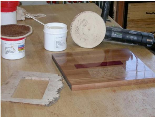
Do the same thing as before - use a stick to spread it evenly over the surface of the felt pad. Then, with the buffer still set to a slow speed, evenly spread this grit over the work piece.
