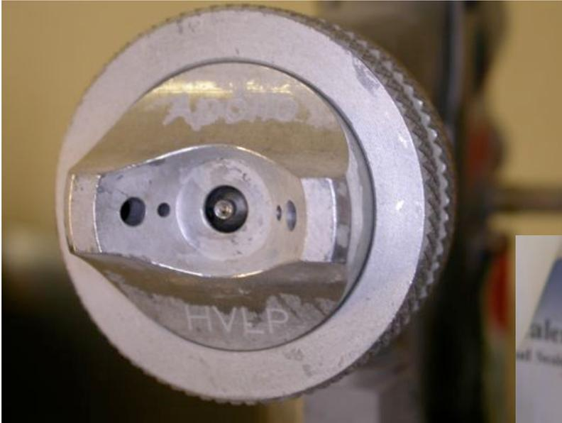
Apollo turbine gun. Around the center of the nozzle is an opening through which the atomization air flows. Contrast this with the Asturo HVLP gun (below) which uses the eight small holes outboard of the nozzle to atomize the air and the Asturo
