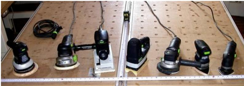
“sanders” that are in use in my studio are shown here. Some move the abrasive in a circular motion like a grinder, some in a linear motion, some in an arc, and some combine various of these to create complex movement patterns, like the so called “random orbit” sanders. The objective is to smooth the surface of the wood while minimizing the scratch marks left behind.
