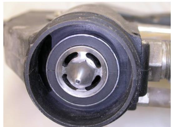
omization air flows through the four center slots. A rubber gasket allows the air cap to seal these two chambers off from one another on the back side.
