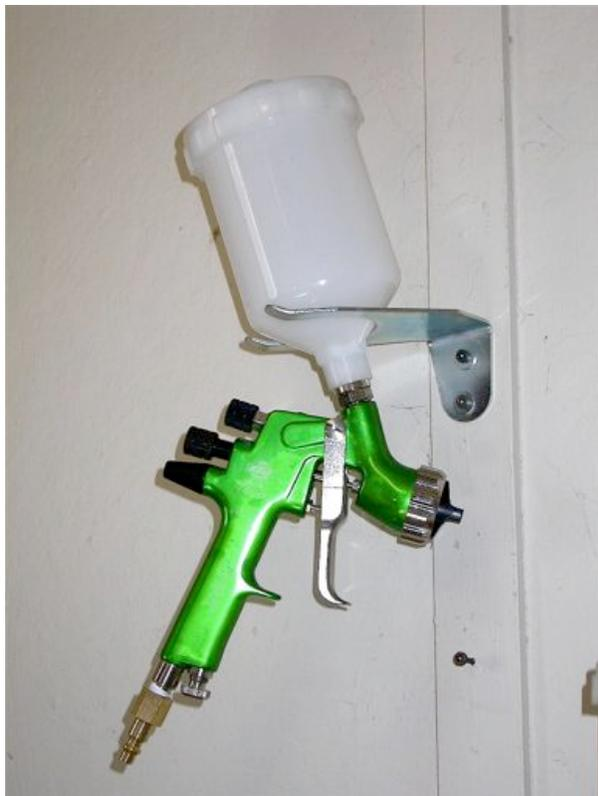
atomization air stream and shapes the fan pattern. These become very important in understanding how the different guns perform in terms of applying finish
