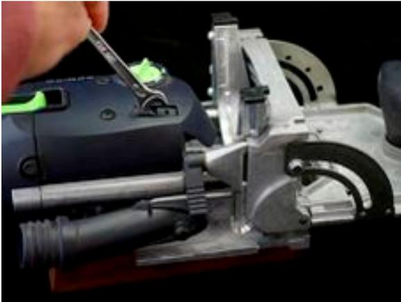
is ideal for this. Hook the edge of the wrench beneath the lock tab and lift it up.
