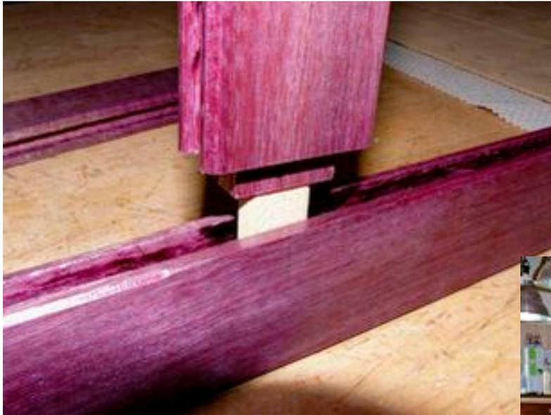
grain component that will attach to the long grain of the back lower stile, we can screw these two together with the screws placed inside the sliding dovetail slot.
