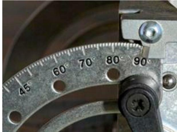
piece (meaning the fence is parallel with the cutter) to zero degrees relative to the edge of the work piece (meaning the cutter is moving perpendicular to the fence the way it is shown in the photo left).
