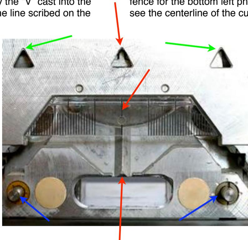
5mm beyond the left end of the rule and the 74mm mark are lines denoting the *outside* edges of the alignment pins.
