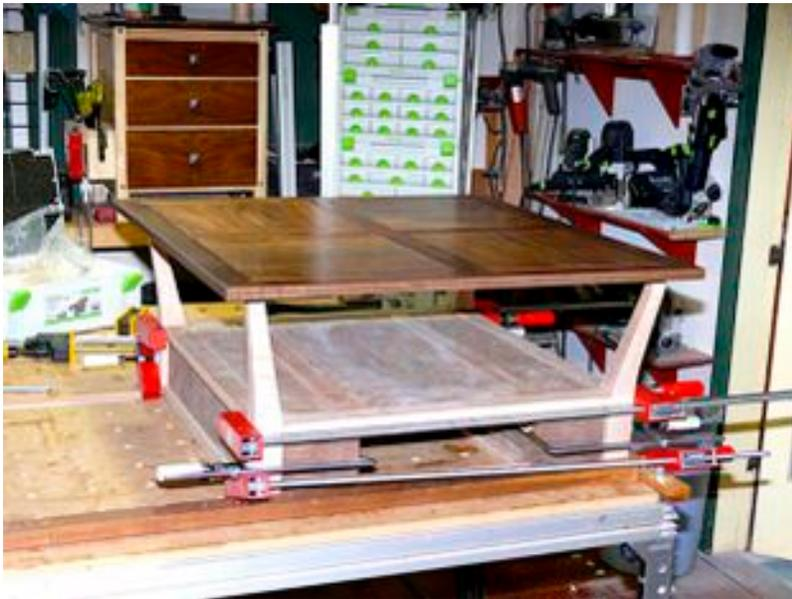
In the upper left photo the top is registered into the end-of-leg to underside of top Domino M&T joints to make sure the legs and top will properly mate in the final assembly.
