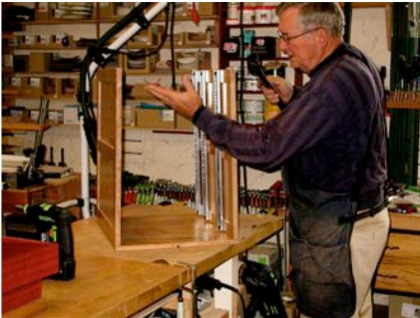
In the lower photo you can see the faux drawer end attached to one side, and below while I am installing the drawer slides.
