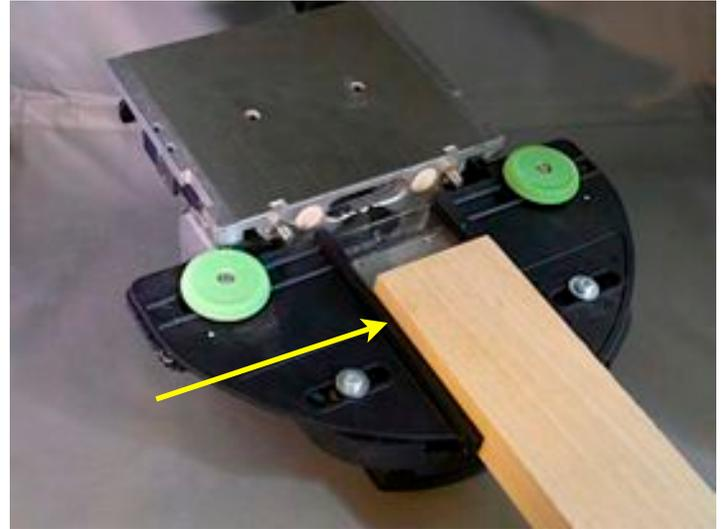
and on top (detail below), is a scale that indicates how far away those fence sides are from the vertical center of the mortise slot.
