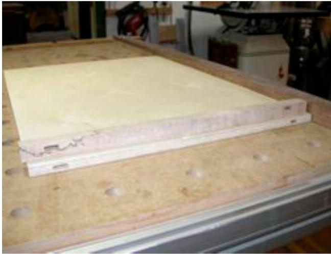
your work piece is wider than that, you can trap the work piece between the face of the Domino and the edge of the top while pushing down on the Domino fence to register and hold the material in place
