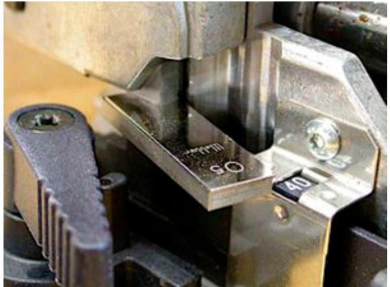
and forth to establish a step that will position the Domino fence up half that amount from the centerline of the cutter. One of those stop block settings is for 40mm thick material and it will position the cutter right in the center, or 20mm up. We need 22.5mm up to center on our 45mm legs, so I placed a 5mm gauge block between the step and the fence to register the fence for a 45mm stock thickness to put the cutter centerline up 22.5mm.
