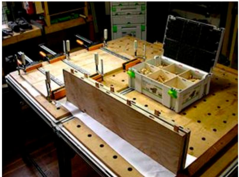
***I suggest you always work with the fence on the top or “good” surface of your work pieces so those faces will align even if the two work pieces are not exactly the same thickness.***
