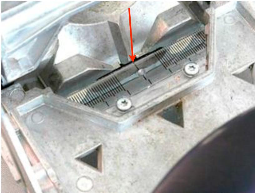
Here is a picture of the guide taken from above the fence when it is lowered to the horizontal position parallel with the bit oscillation. In use, it is quite visible and I am constantly impressed by just how close I can set the Domino mortise slot with just this visual reference.
