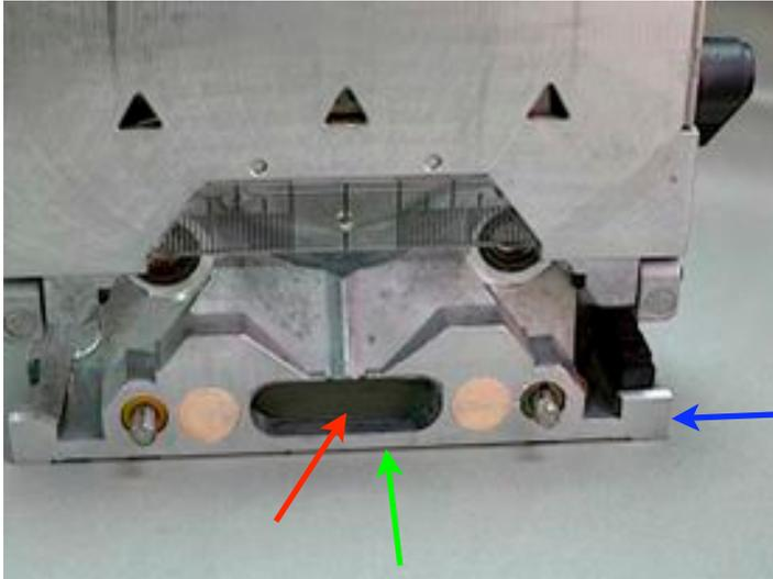
emerges when the body is pushed towards the work piece to make the mortise cut. **The cutter centerline is 10mm up from the base of the fence assembly (green arrow above).**
