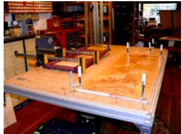
In the photo above notice how handy the Festool DX 93 E detail sander is for reaching into tight spots such as where the leg stretchers meet the legs. Any glue squeeze out on purple heart really shows once the finish goes on so be sure to sand very thoroughly.
