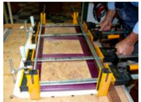
The self-aligning feature of a Domino M&T joint cut inside a normal R&S tongue and groove joint really speeds up the process of assembling a multi-panel component like the back on this piece.
