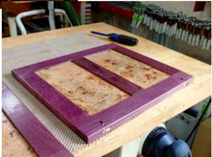
Now let's revisit the sliding doors. Earlier I said that the doors had to fit snugly into the door openings to look right. The problem with most sliding doors is they have to fit loosely enough to lift up into a top track to let the bottom free of the bottom track to get the doors in and out. That simply looks bad and is not pleasing to use.
