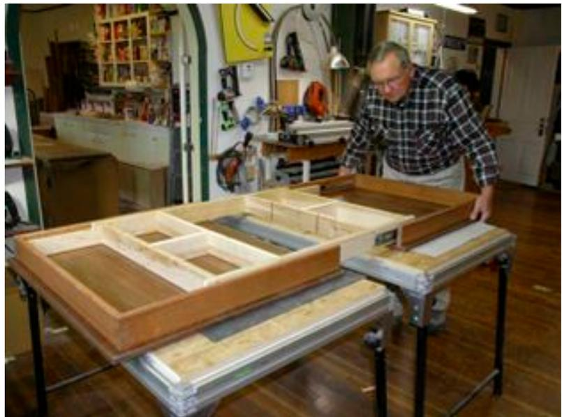
The frame is a simple box section made up of two side rails the same as the net
