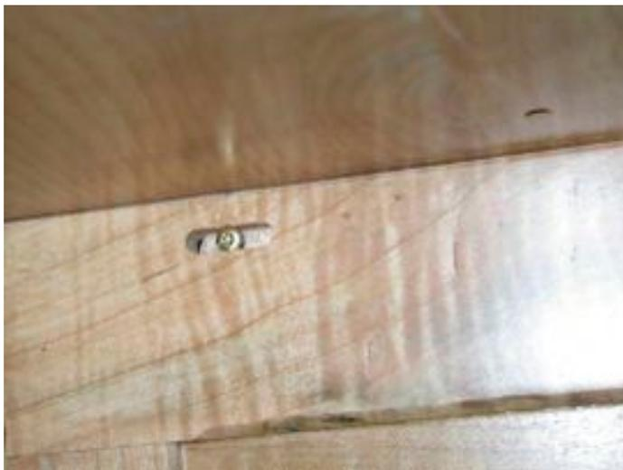
front to expand and contract independently. You could also use a dowel to pin the tenon, but the screw is faster.
