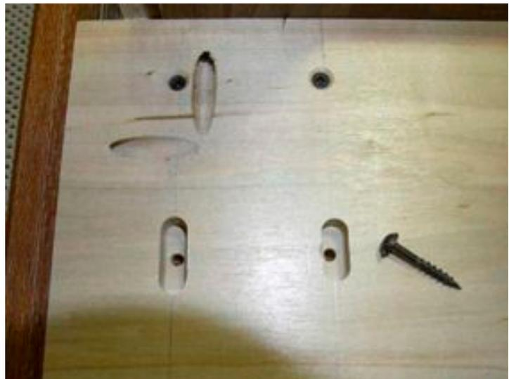
Before we move on we have to remember that the maple top plate itself is a piece of solid wood, so we need to accommodate its natural wide grain movement as well.
