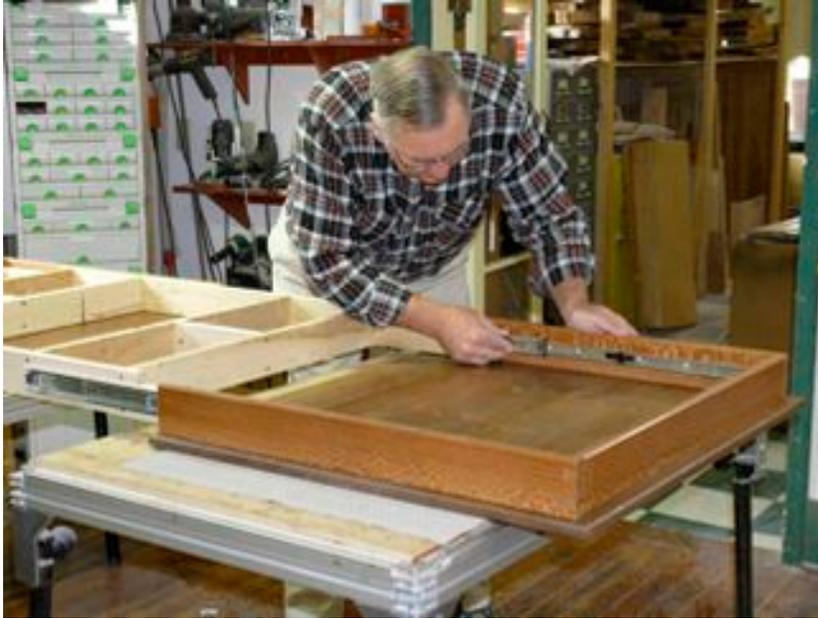
Note in the lower photo how I am using two Festool MFTs, each with a rubber pad protecting the finished top surface, to slide the whole thing together. I am moving the MFTs with the skirt/top assembly held stationary so I don't scratch the beautiful top.
