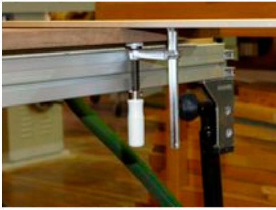
clamp a long Festool guide rail parallel with my intended line of cut for the sliding dovetail slots that will hold the side skirts (photo above).
