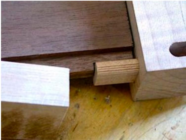
ino tenon since the centerline of the tenon and the bottom of the dado are both 10mm. (Suppose we should invent a term and call this a “Dominoed dado” joint? grin.)
