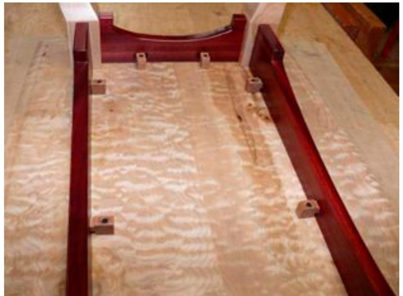
You can also cut these mortises from the top side if you want more bottom of slot to underside of top dimension. Set the Domino fence height to wherever you want the center of the slot. Add on the auxiliary base for stability. Place the fence on the top edge of the skirt with the auxiliary fence held to the inside face of the skirt and make the cuts. Machine tongue blocks to match, screw them
