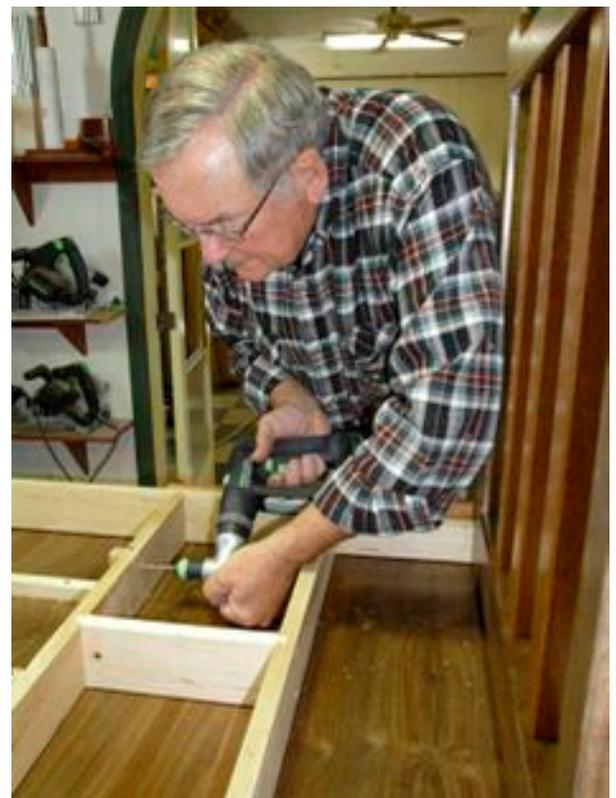
Once you also add the leaf guide pad assembly, use screws to pin these dovetails in place and you are nearly done. Notice how handy the Festool right angle attachment for the drill is in getting into the tight recesses of the frame.
