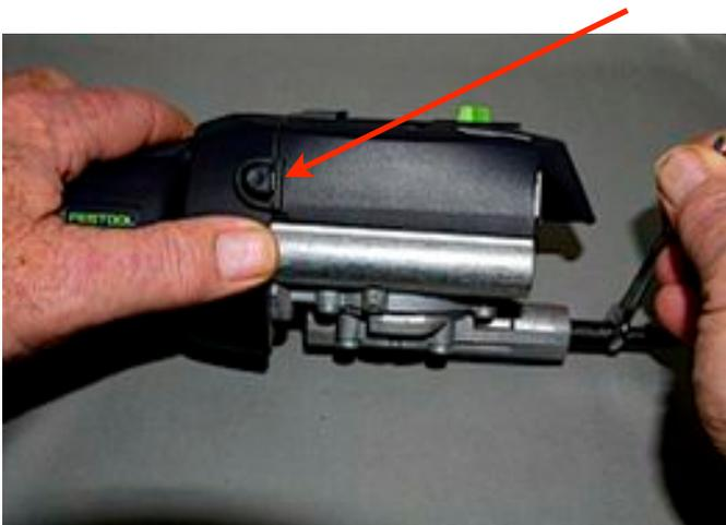
other hand. In the photo above I moved my thumb down so you can see the shaft lock lever (red arrow).
