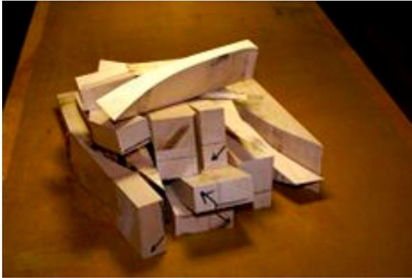
Sand all the legs to final shape and dimension and cut the profile for the skirts. I like to break the edges on things like skirts with a 45 degree chamfer router bit so the hand feels a smooth, rather than a sharp edge.
