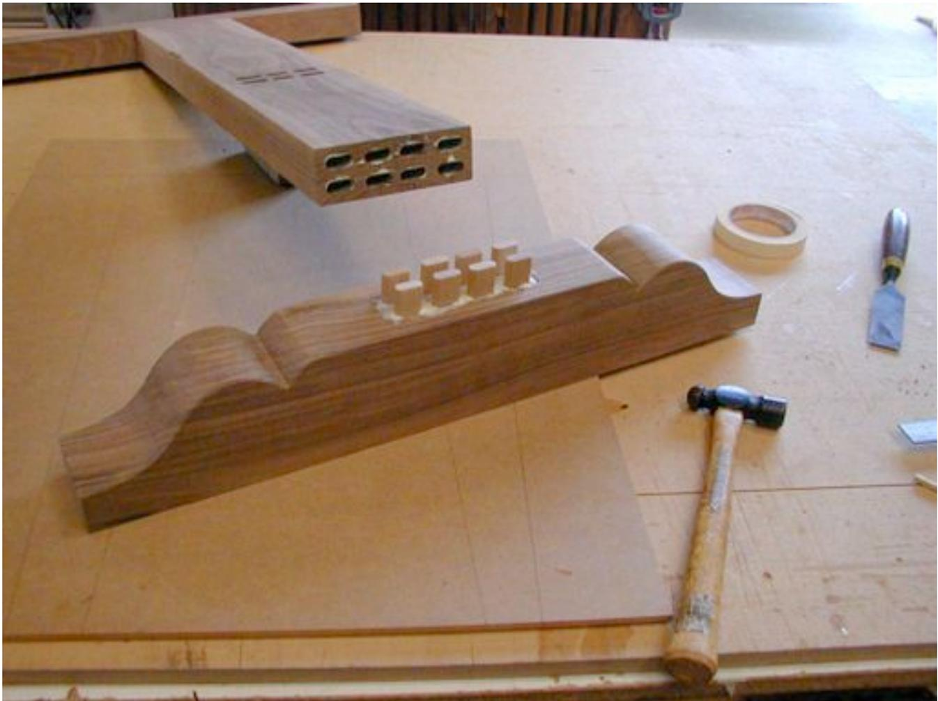
This photo (supplied by Festool) shows one example. The leg to base joint uses eight Dominos stacked in a 2 x 4 array while the leg to stretcher joint uses six Dominos stacked in a 2 x 3 array.
