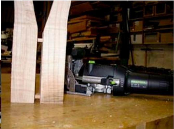
fence to one-half the leg thickness so the leg will snugly fit inside the saddle fence. Then I slide the Domino machine up until my mark is aligned with the mortise centerline on the Domino machine fence. Then the clamp
