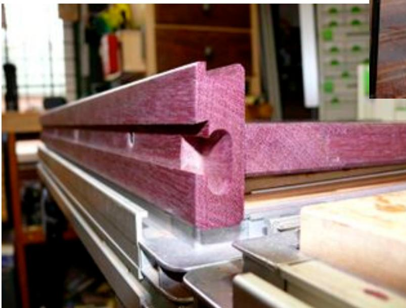
between the two leg stretchers using Domino tenons inserted dry (no glue) into wide mortises cut on the inside of the stretchers and the ends of the shelf. From previous descriptions, aligning these
