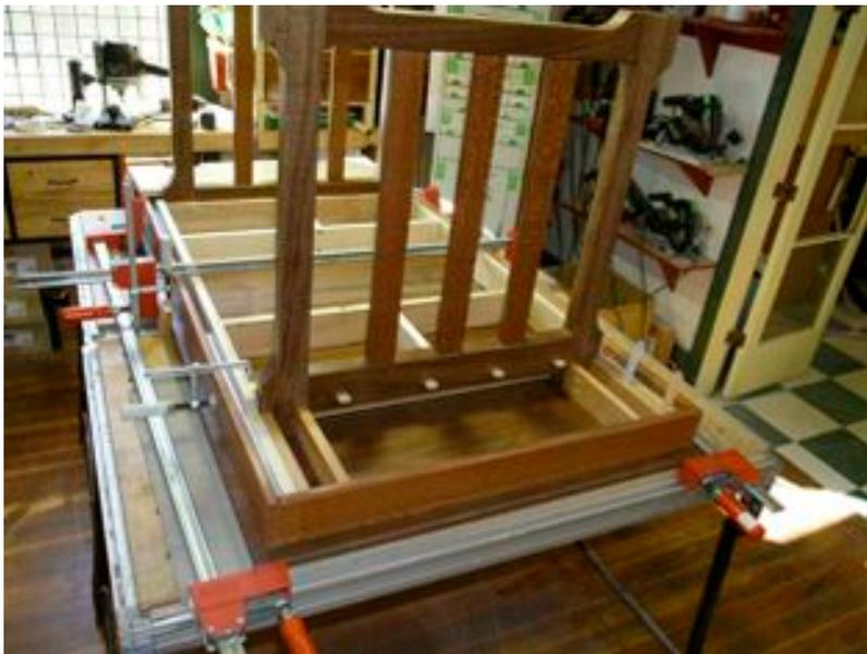
A maple top plate is then Domino mortised and tenoned into the leg holding the maple top plate flush with the top of the fillers and secure to the face of the leg. The plate is then screwed down tightly to the fillers. The underside of the top forms one side of a torsion box, while the maple top plate forms the other side. The fillers hold these two apart and act like an "I" beam spreading the rack
