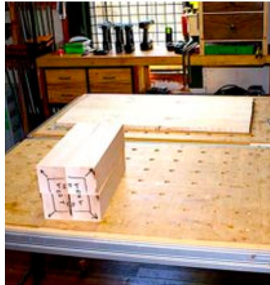
the outline of the square top of the leg on each block and draw an arrow pointing diagonally out to what will be the outside of the cabrio curved leg.
