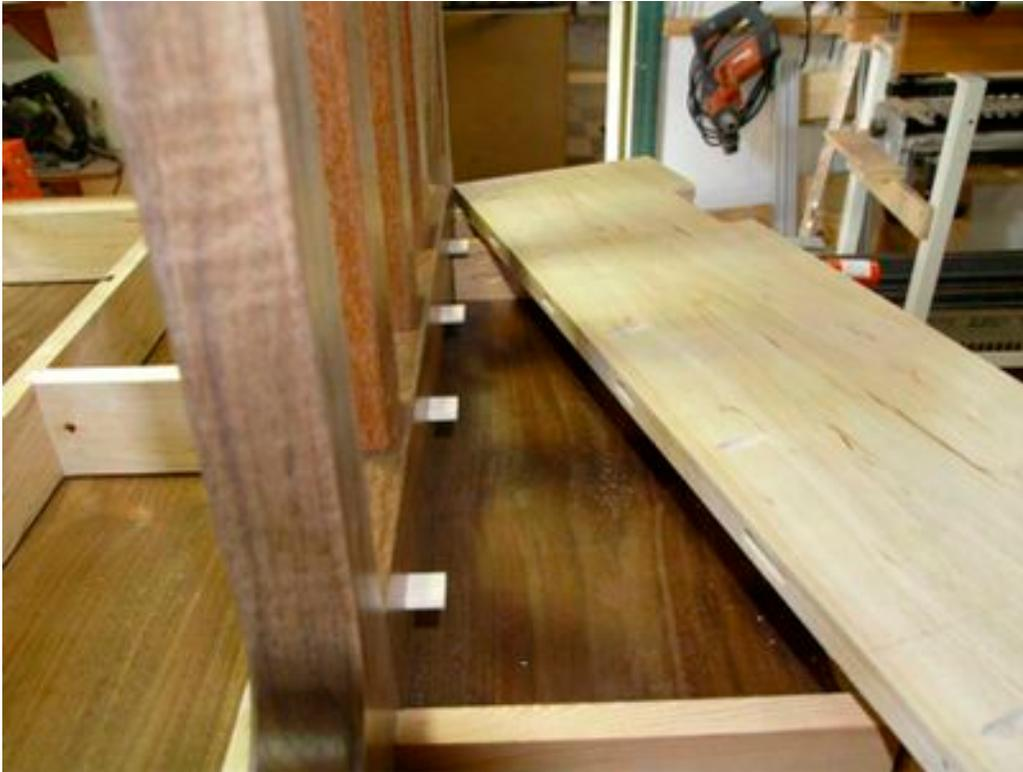
This is easily done with a neat Domino “trick.” Drill the through holes to be larger than the diameter of the attachment screws. Center a Domino mortise about 5mm to 10mm deep on those attachment holes as shown here. If the maple top plate wide grain moves relative to the long grain of the torsion box fillers, it can slide in the over-
