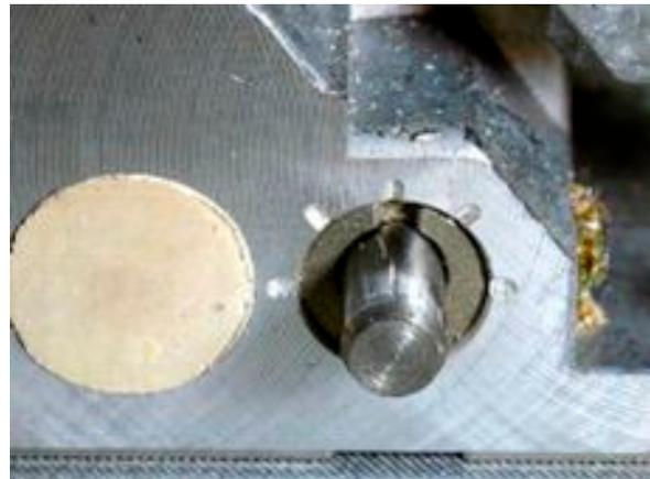
The vertical centerline of the cutter is also marked in several other ways (red arrows) as well: by the "V" cast into the fence base, by the line scribed on the clear plastic reference scale attached to the moving portion of the fence (note the hole in the plastic denoting center), and the point of the triangle cast into the moving portion of the fence.
