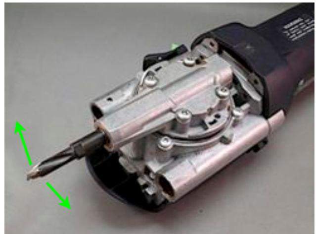
Here is a view of the under side of the body. The round housing held by the four screws is gear driven to move the cutter tip back and forth in a horizontal arc while the cutter is also rotated to make the cut.
