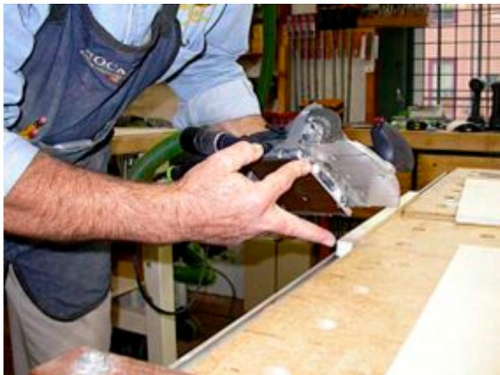
your work piece is wider than that, you can trap the work piece between the face of the Domino and the edge of the top while pushing down on the Domino fence to register and hold the material in place
