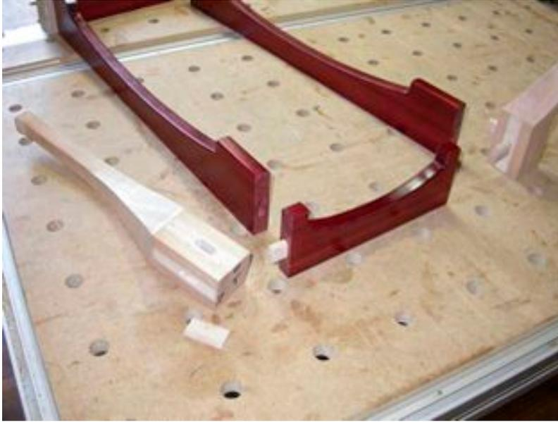
It is easy to make a tongue block with the base of the tongue up slightly less than 7mm from stock that is 12mm thick. That will present a 5mm tongue to insert into the 6mm slot cut on the inside of the skirts. By keeping the bottom of the tongue a bit less than 7mm, when you screw that block to the underside of the table top the tongue will press the skirt firmly to the top while still allowing it to move with normal seasonal changes in humidity.
