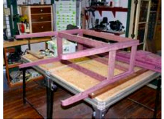
These are the main pieces of the skeleton. Note that the top edge of the front, back and side frame members all align with the top of the legs. The lower edge of the front, back and side frame members align together.
