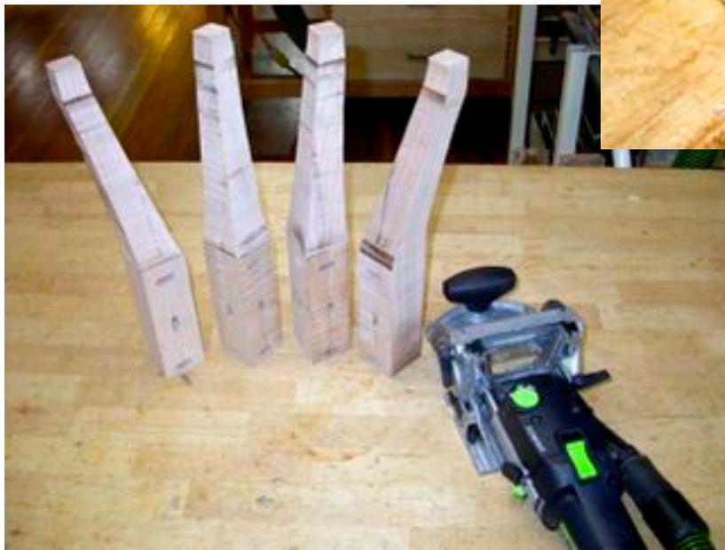
we need three Domino mortises on each of two sides of each of four legs. The upper and lower horizontal mortises will attach the legs to the platform frames while the vertical mortise will attach the skirts to the legs.
