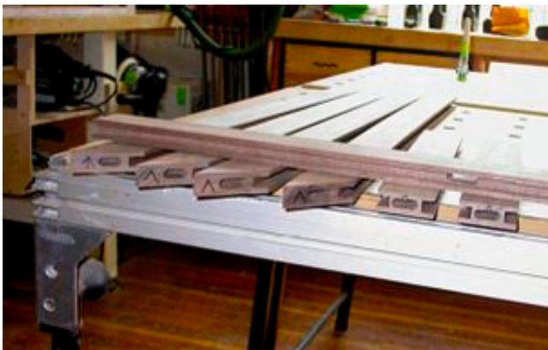
square to establish the length I wanted each mortise to be down from the outside edge of the 45 degree frame corner and used that to make a mark on both ends of the four frame members.
