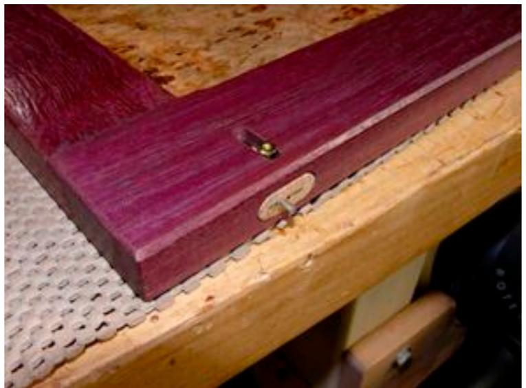
smaller in diameter than the width of the sliding door tracks machined in the front upper and lower frame members. I cut the length of the tenon so the end of the pin would be flush with the bottom or top surface of the door when it was fully inserted into the 10mm mortise. A hole was then drilled into the face of the 10mm tenon through the center of the 5mm mortise so a small screw can secure the 10mm tenon/pin unit either withdrawn up into the door or with it low-
