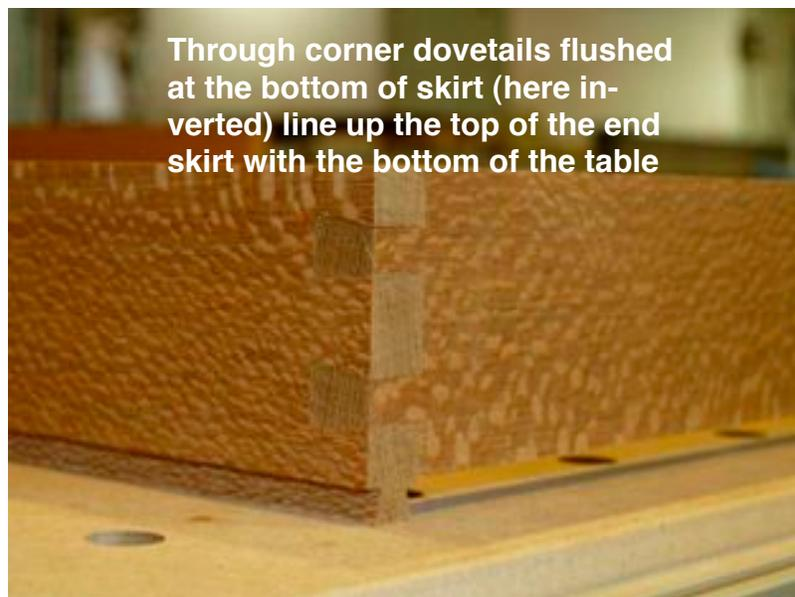
**Through corner dovetails flushed at the bottom of skirt (here inverted) line up the top of the end skirt with the bottom of the table**
