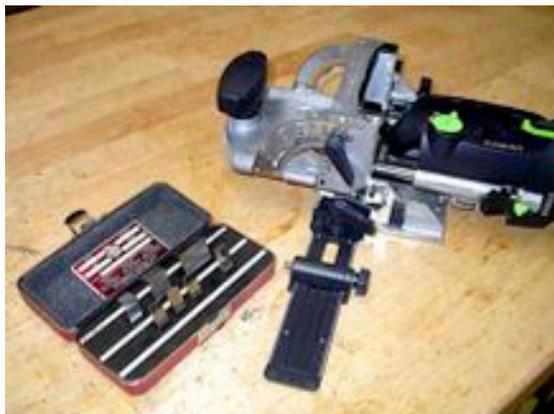
the Domino fence to be exactly 22.5mm to center those on the 45mm thickness of the legs. They must be spot on because those skirts will sit in a dado we will cut in the platform frames and they have to also index into the legs via these Domino M&T joints.
