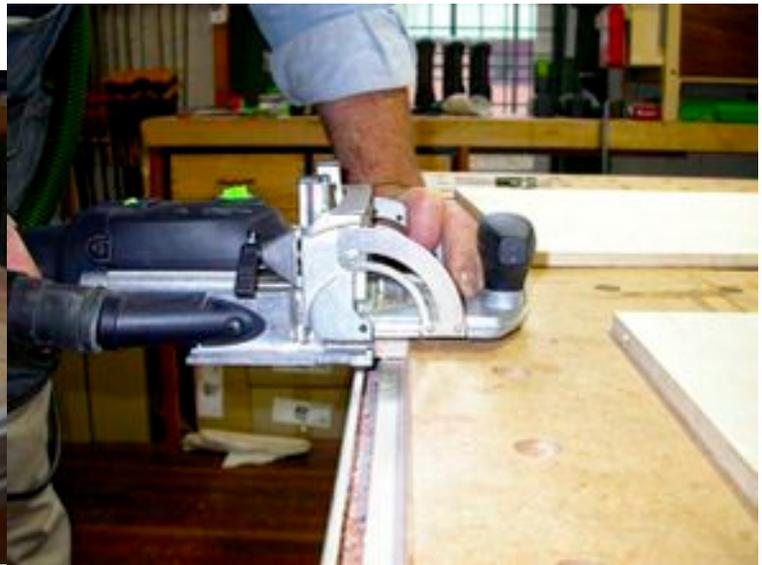
while you cut the mortise. I also like to register the end of the piece against a stop so it can't slide side to side while I am making the cuts, especially if I am using one of the spring loaded pins for end to mortise registration as I am doing in this example.
