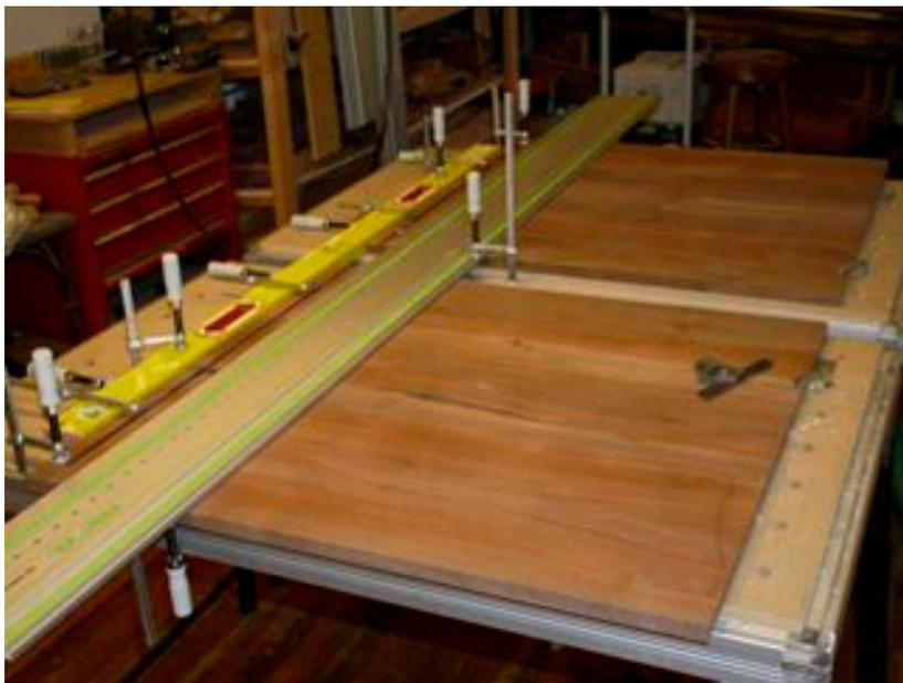
assembly to the exact same width as you cut each top plate making sure it is also very square edge to side.
