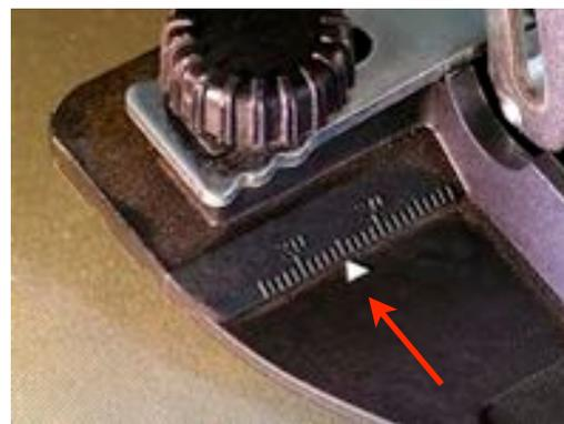
piece? Set the fence to 10mm high and set the two sides of the saddle fence to 25mm as shown above. The resulting mortise will be exactly centered in the
