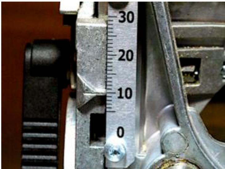
The stop block (shown here at a setting of 20mm) is marked in units corresponding to the **overall thickness of the work piece for which the cutter will be exactly centered**. In this case the stop block is set for a 20mm thick work piece resulting in the pointer (photo left) indicating that the centerline of the cutter will be at 10mm.
