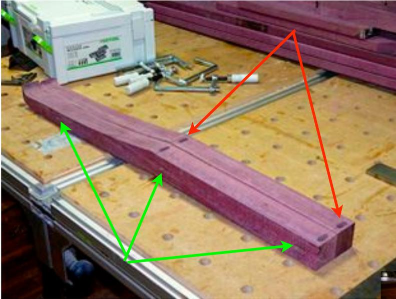
and lower side frame members and to hold the leg stretchers. Since those frame members are oriented with their wide face up and down (where the front and rear frame members are oriented with their narrow edge up and down) we need to cut those mortises in a vertical, rather than horizontal orientation as shown below.
