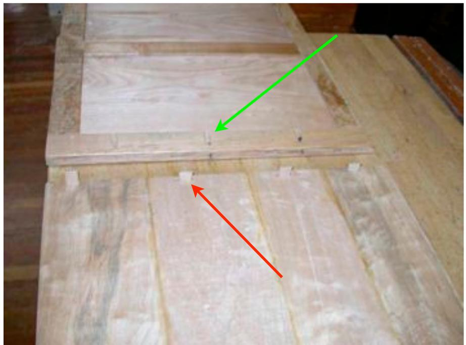
by one or two Domino placed along the thickness of the edge, it is good practice to stack Dominos using multiple sets in the same joint.
