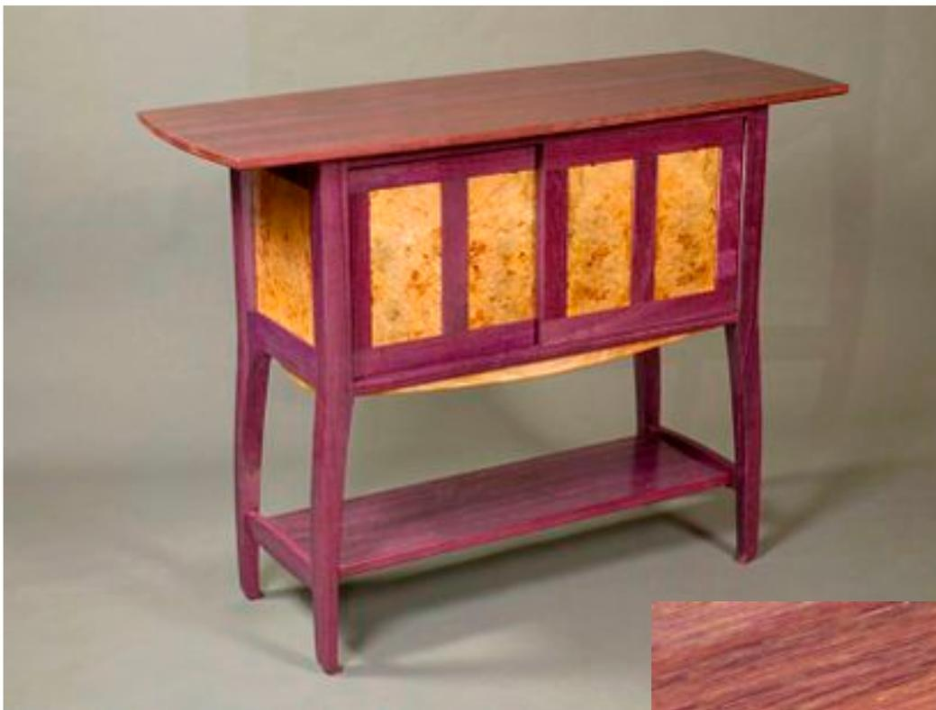
the legs and upper frame by tongued splines screwed to the underside of the top. The bottom shelf is held to the leg stretchers by wide Domino mortise slots and tenons inserted without glue to allow for seasonal expansion and contraction of the shelf.
