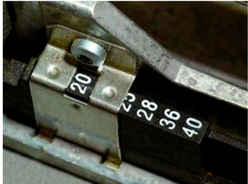
The first adjustment to consider is the height the fence is above the **horizontal centerline** of the cutter. That is shown by a scale and pointer. In the close up photo below the fence is set to be exactly
