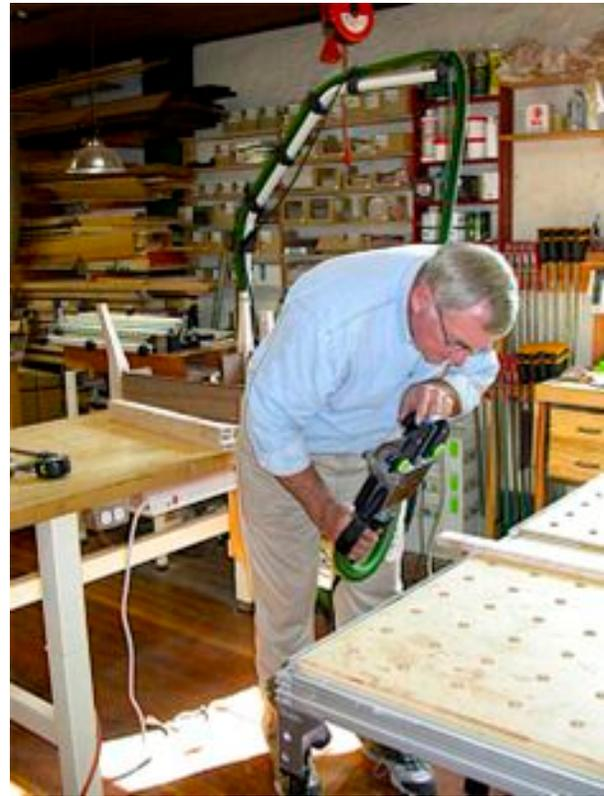
In these photos you can see the Domino machine with the saddle fences set for the 50mm width of the platform frame members and the fence set to center the Domino mortise on the 20mm thickness of those pieces.
