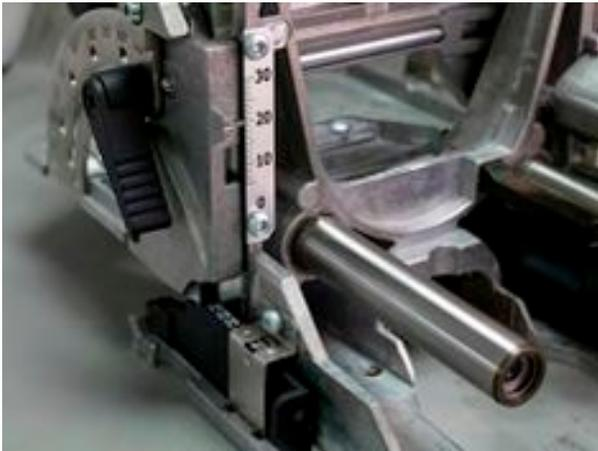
10mm above the centerline of the cutter. A lock lever secures the fence at the desired height. The fence moves up and down on machined ways so it remains exactly parallel with the cutter at all heights.
