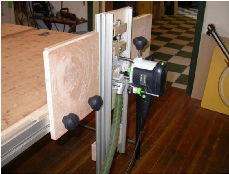
and bottom pieces establish and hold the distance between the two aluminum rails to be the same throughout the range of travel of the center, router base, component. Adjustment is easy, smooth and very repeatable. No locking is necessary since the weight of the router holds the setting well.
