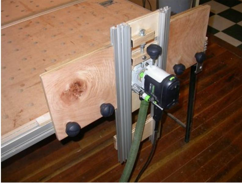
The jig is constructed from standard Festool catalog MFT rail pieces, Festool knobs and hardwood plywood scraps. The MFT rail sections form both the structure for the jig and guide the router base plate while it is raised or lowered to expose more or less of the dovetail bit.
