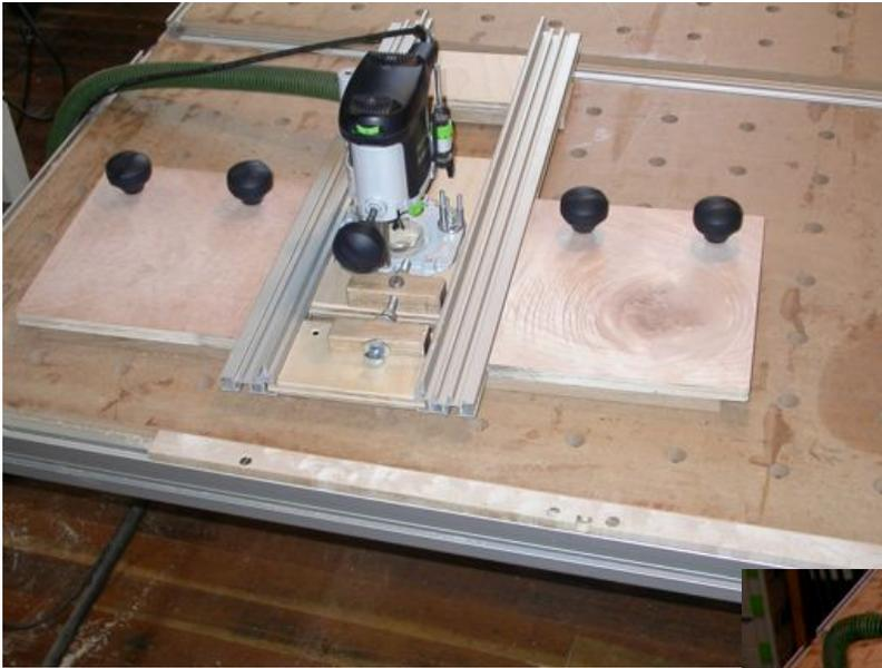
This photo shows the completed unit resting on top of a Festool MFT with a Festool 1010 router attached. The fence base is shown held to the top of the MFT side rail by recessed 8mm flat head screws threaded into nuts in the top “T” slot on the MFT side rail.
