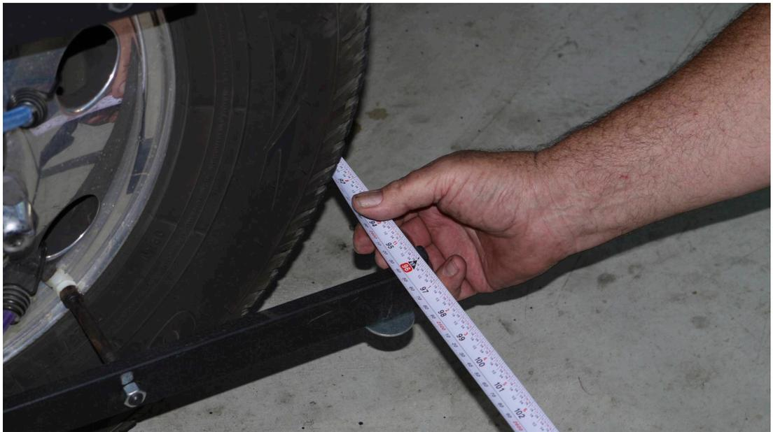
Ideally you will want to adjust the tie rods on both wheels by the same amount until the total toe is close to zero.
