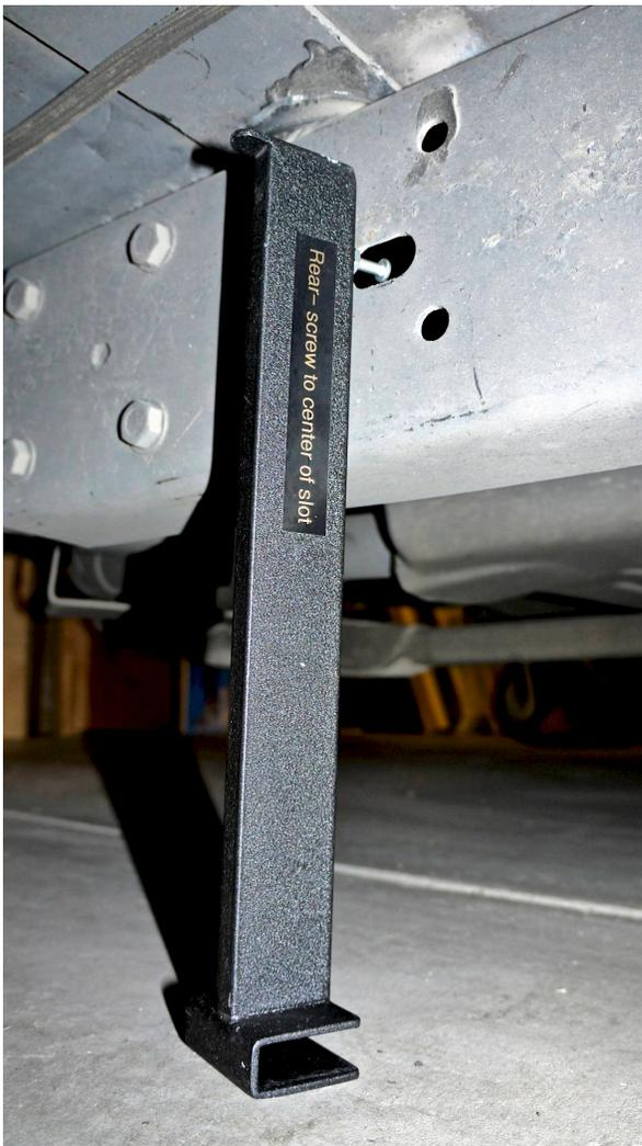
Since the rear ride height slot on the driver's side was removed on most coaches to make room for the generator, you need to measure from the ground to a known spot on the passenger side in order to check the driver's side rear ride height. Add or subtract air in the driver's side air bag to match the measurement you took on the passenger side.
