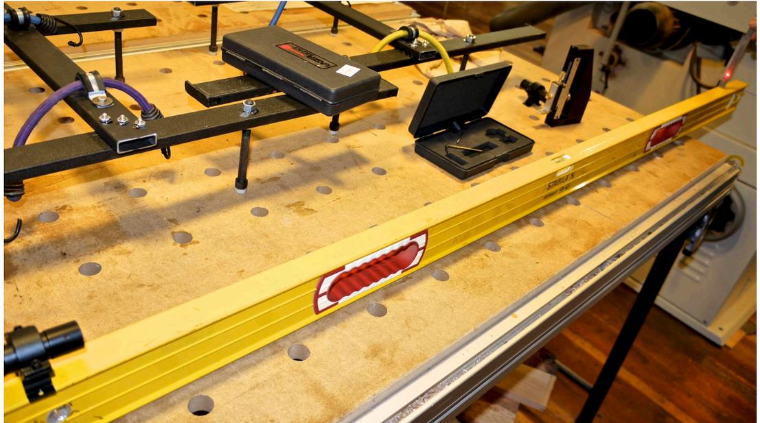
I used a long Stabila level and a metric rule to set the beam true to the mount and then rechecked it again once the units were mounted to the insides of the lower arms as shown in the photo below.
