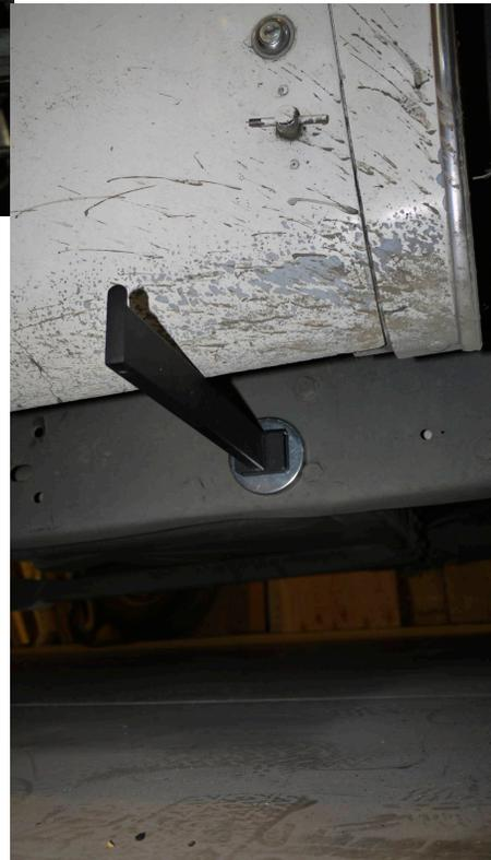
target to the front and see if the laser hits the same line on the target. If not, move the steering wheel one half the difference and recheck. When the laser hits close to the same line on the target
