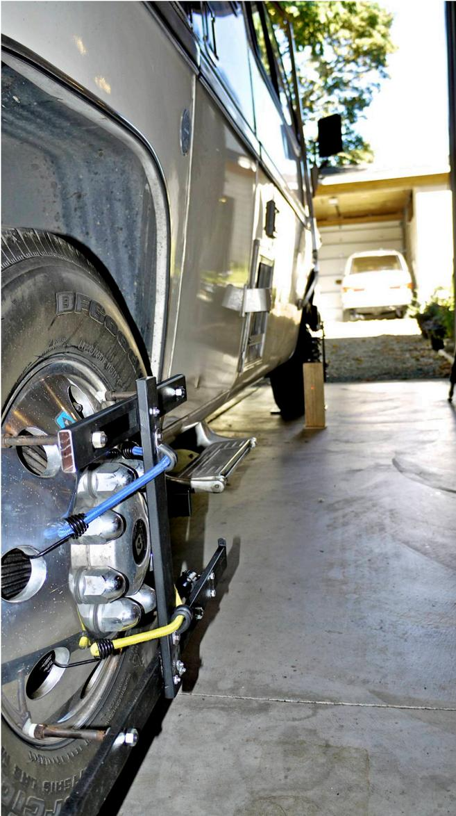
Repeat this process on the middle bogie wheel on that side. This will give you camber and parallelism on both bogies on that side.
