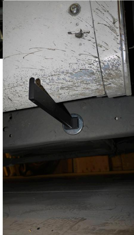
My coach has the front wheels spaced out to be even with the rear wheels as part of the one ton front end conversion. If yours are in the stock configuration, you will need to slide the laser target further inward matching a line on the target with the end of the magnetic stand-off arms to make your readings. If you are making your own kit you can also mount the lasers to the outside of the lower arm so it will hit the target when the target is against the outside of the stand-off arms.
