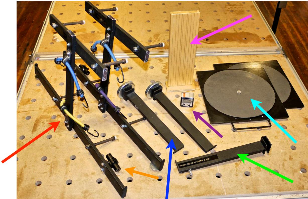
There are only nine parts to the kit - two bungee cord attached stand-off plates (red arrow) each with a gun sight laser mounted to the inside of the lower arms (orange arrow), two magnetically attached laser target stand-off arms (blue arrow), two turntables (cyan arrow), a go/no-go ride height gauge (green arrow), a laser target (magenta arrow) and a digital angle meter (purple arrow).
