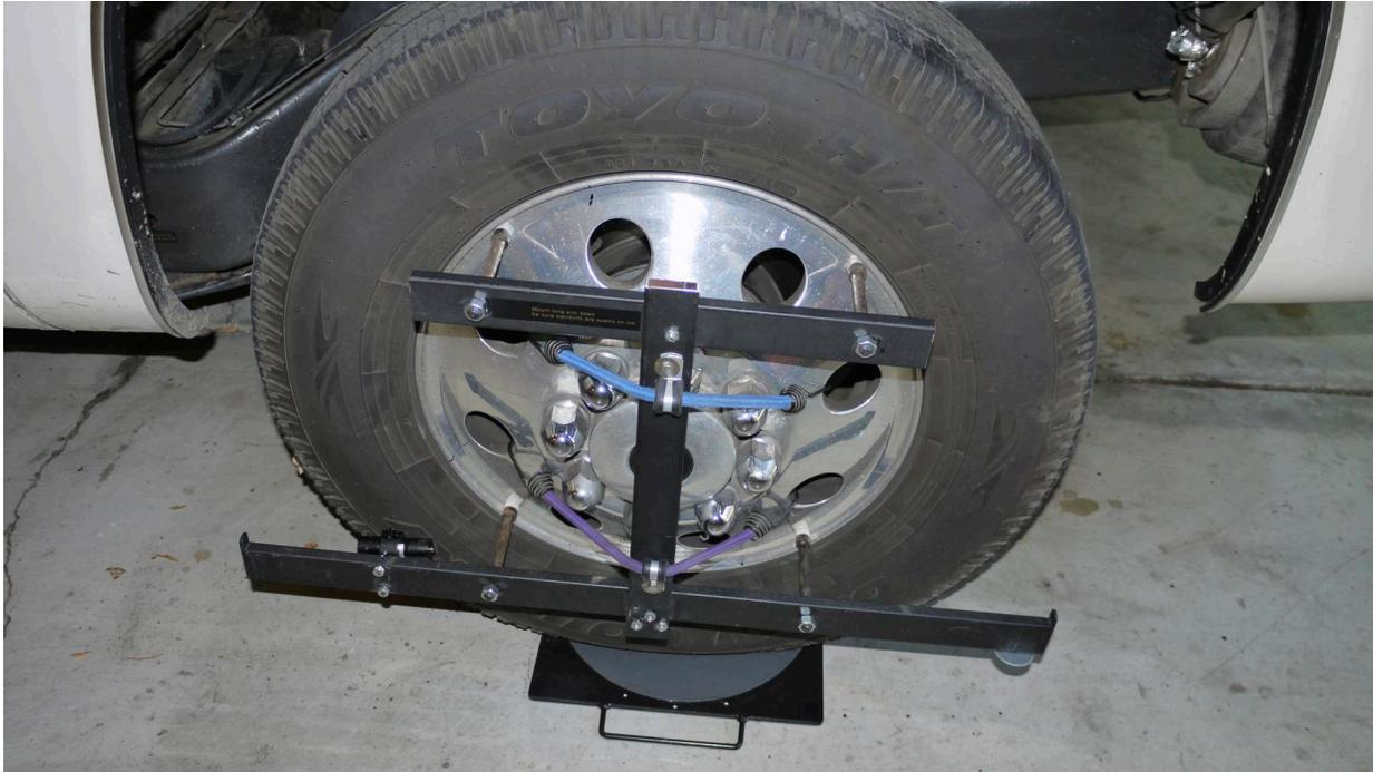
Place the now zeroed angle meter on top of the long arm and gently move the stand-off assembly to level the lower arm. That will also insure the upright member is exactly at 90 degrees to the parking pad surface.
