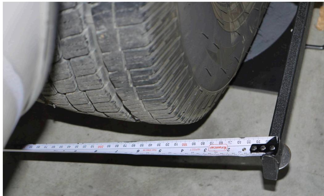
Once the wheels are pointing straight ahead, put one end of a tape measure on top of the end of the lower stand-off arm and measure to the same end of the lower stand-off arm on the
