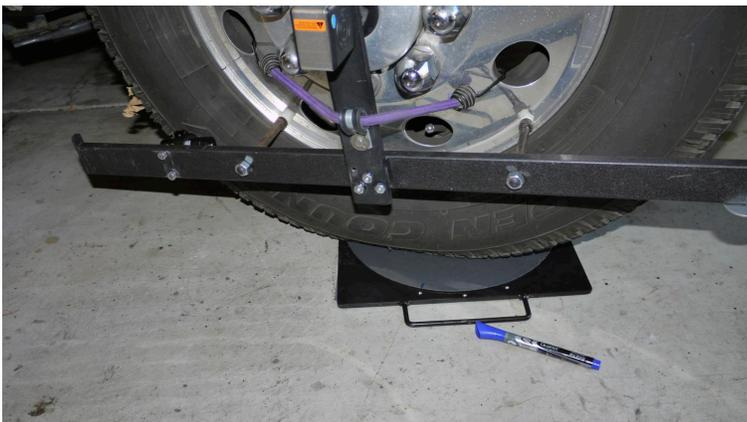
To accurately determine when the front wheels are pointed straight ahead requires a way to measure the plane of the rim and how that relates to the frame of the coach. The plane
