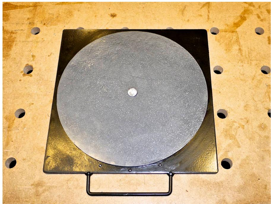
is no index mark on the round sheet. Once the coach is rolled up on these turntables a mark with a dry erase marker provides the reference required to reliably hit 20 degrees each way to do the camber calculation. These are simple, require little or no maintenance and should stand up well to rough handling by many users.
