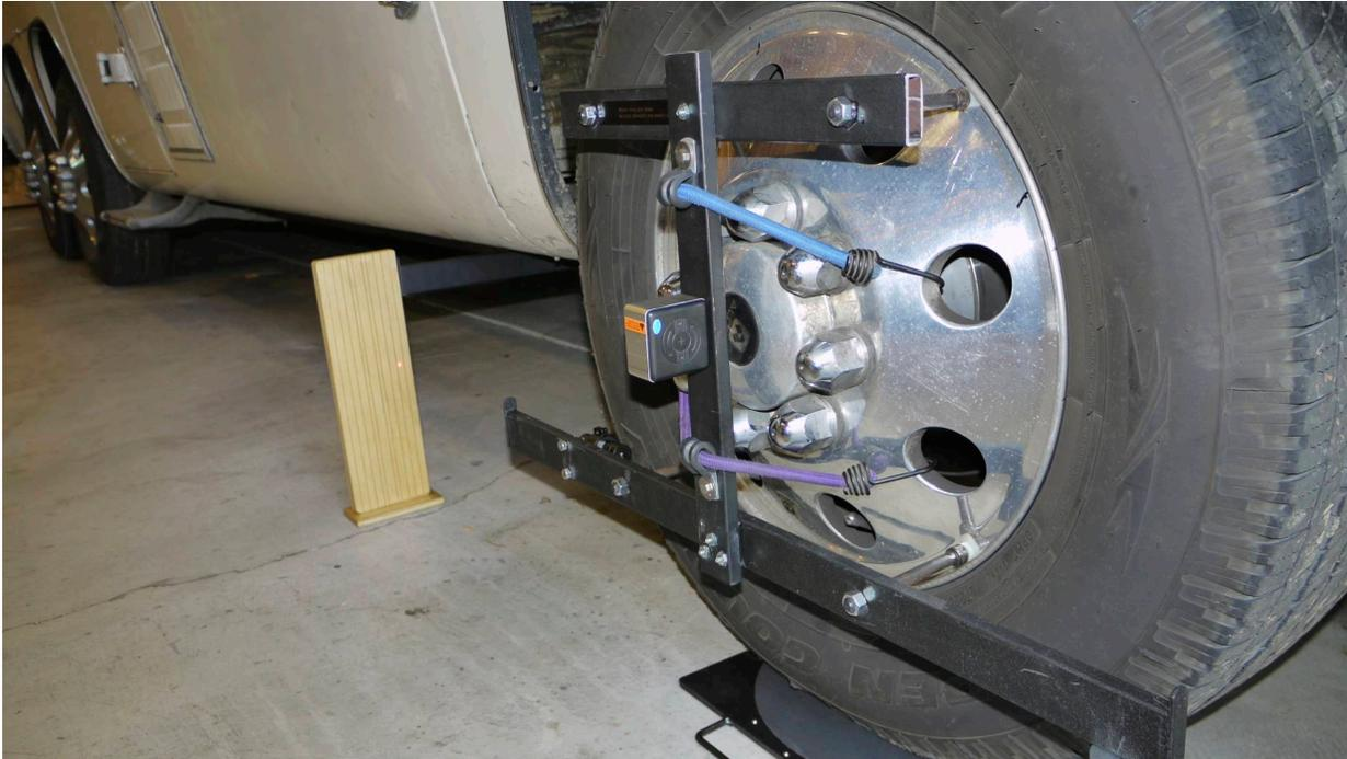
At the rear we need to make sure all four bogie wheels are running parallel with the frame and that all have about one degree of negative camber when the coach is settled in at proper ride height.
