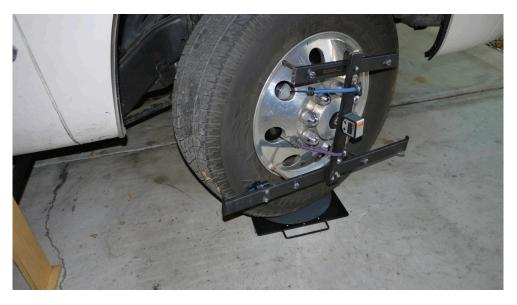
*Multiply this camber change reading by 1.43 to calculate the caster angle on that wheel.* Record that amount.
