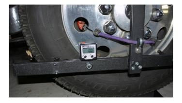
Magnetically attach the laser target stand-off arms to the frame front and rear near the ride height measuring slots. Place the
