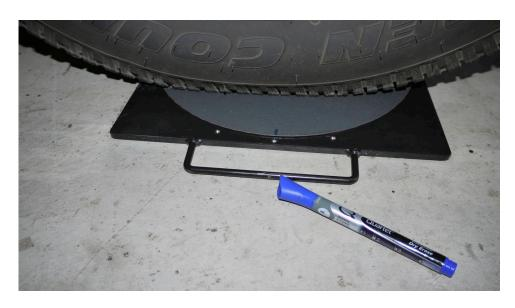
plate. This will allow you to precisely turn the front wheel 20 degrees in each direction in order to calculate the caster angle.
