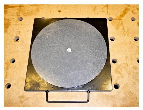
plate and the sheet allow easy movement. The tire sits on the round sheet which rotates as the wheel is turned. Index marks on the plate show zero and 20 degrees each way. There
