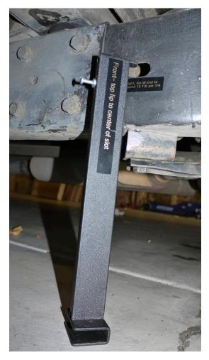
miles to allow the suspension to fully settle in before you measure ride height again.
