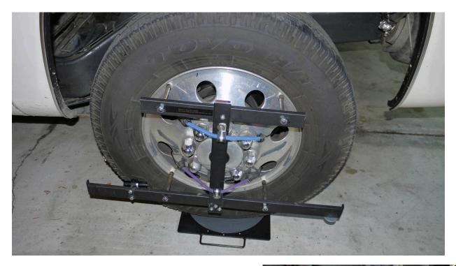
Place the now zeroed angle meter on top of the long arm and gently move the stand-off assembly to level the lower arm. That will also insure the upright member is exactly at 90 degrees to the parking pad surface.
