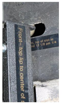
If the front ride height is off when the rear is correct, the only way to change the front is to adjust the front torsion bars. That REQUIRES the use of a special torsion bar unloading tool while the coach is jacked up and the knowledge to follow all the necessary safety procedures.
