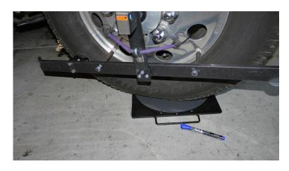
type turntables won't work well for our GMC motorcoaches. We need turntables that are no more than 1/2" thick so the coach can be pushed or driven onto them without lifting the tires off the ground or overly affecting ride height for all the reasons covered in the section above.
