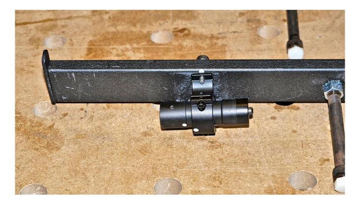
Once the beam was adjusted to be quite parallel to the mount, I put two white paint dots, one on the laser body and the other on the mount so the user can tell visually whether or not the laser has been knocked out of parallel.
