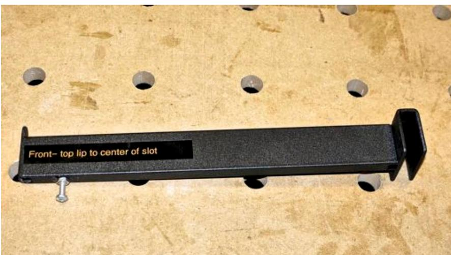
Flip this gauge over and measure up from the bottom 11 5/16". This will be the center of the rear ride height frame slot. Add another tang or screw at this location as well. Now you have an easy to use go/no-go gauge that tells you with unerring accuracy whether your coach is set to the factory ride height or not.
