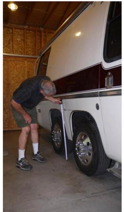
The parallax in the photo right makes it appear that the ride height is too low. It is actually right on as you can see in this close-up photo since the top tang fits inside the slot.
