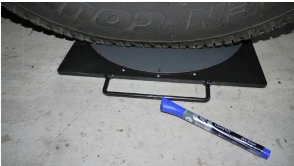
Note the three rivet heads on the turntable base plate. They are set to be 20 degrees from each other. The dry erase marker provided will wipe off when you are through.
