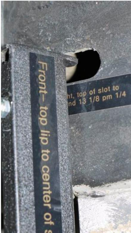
If the front ride height is off when the rear is correct, the only way to change the front is to adjust the front torsion bars. That **REQUIRES** the use of a special torsion bar unloading tool while the coach is jacked up and the knowledge to follow all the necessary safety procedures.
