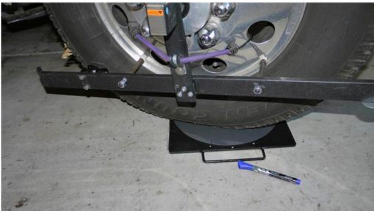
To be able to reliably turn the front wheels the precise 20 degrees both ways requires the use of a turntable with angle measurement indicators. Most commercially available turntables are thick to accommodate ball bearings and side to side movement so require lifting the front
