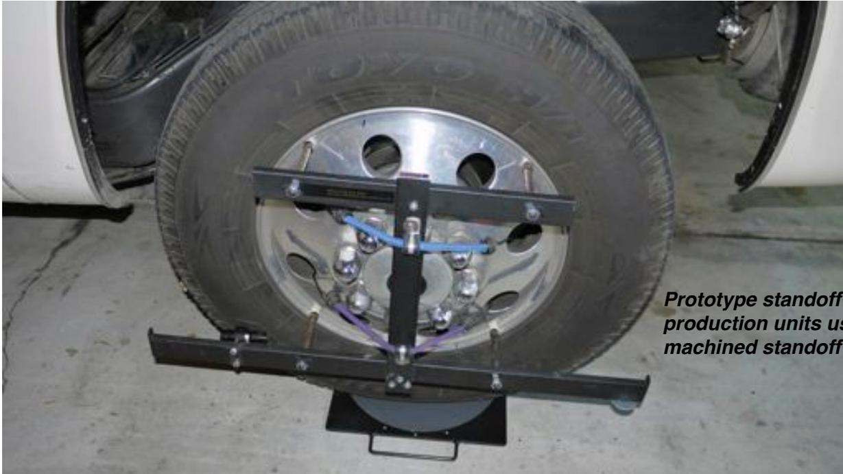
*Prototype standoff plates shown, production units use precision machined standoff pins.*
