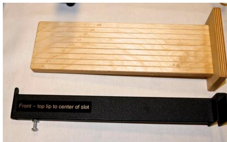
There are two black metal magnetically mounted **frame stand off laser target arms** included with your kit. Follow the instructions to mount these to the frame near the front and rear of the coach.
