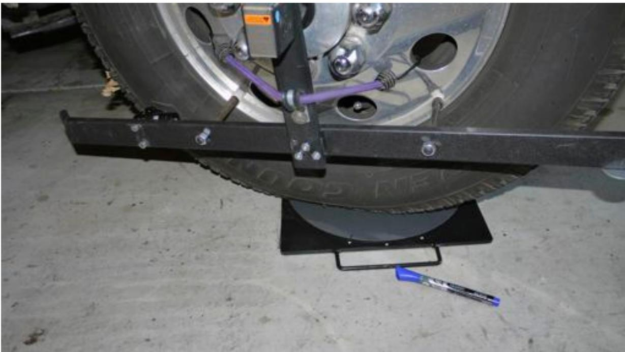
generally return to center a bit on its own, usually leaving the wheels at about the 20 degree point. Turn the wheel a bit by hand to get as close to 20 degrees as you can.
