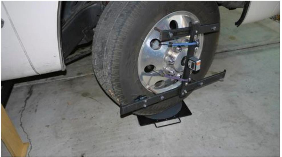
***Multiply this camber change reading by 1.43 to calculate the caster angle on that wheel. Record that amount.***
