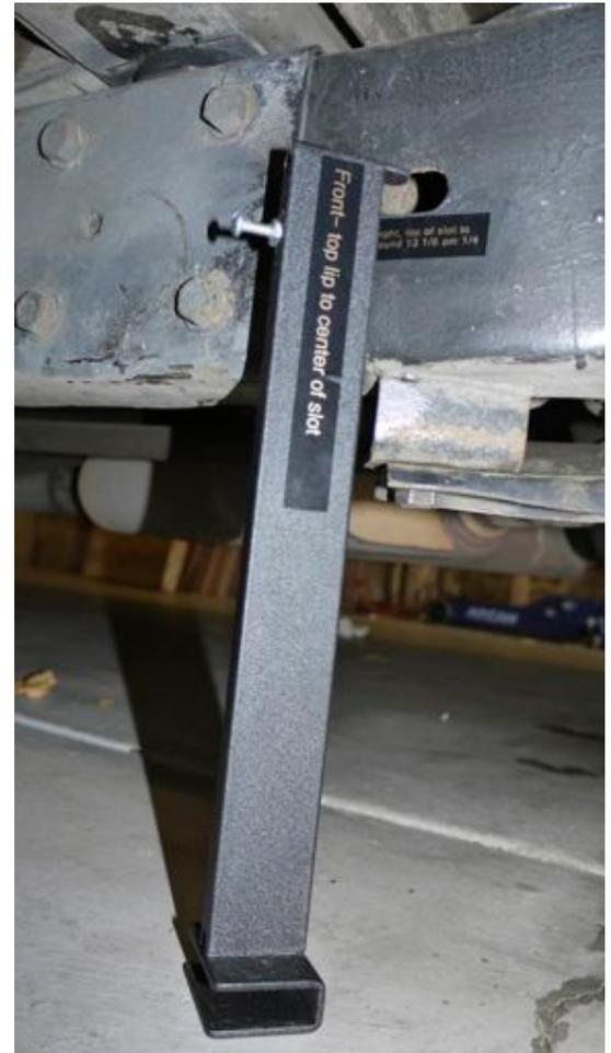
If you do adjust the front torsion bars, drive the coach at least five to ten miles to allow the suspension to fully settle in before you measure ride height again.
