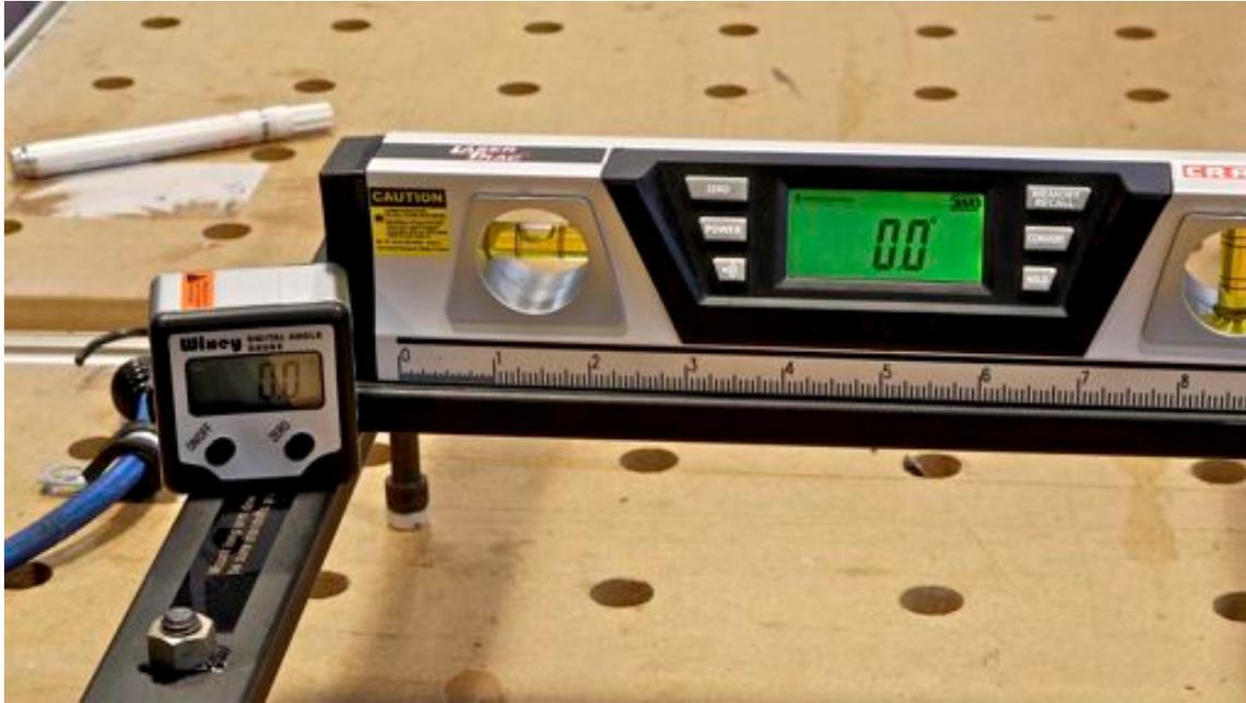
While I found the back lit Sears unit to be easier to read, it was also large enough to be awkward on my stand-off plates requiring the bungee holders to be mounted to the back of the vertical member where they were less effective in holding the stand-off plates securely to the rims as shown
