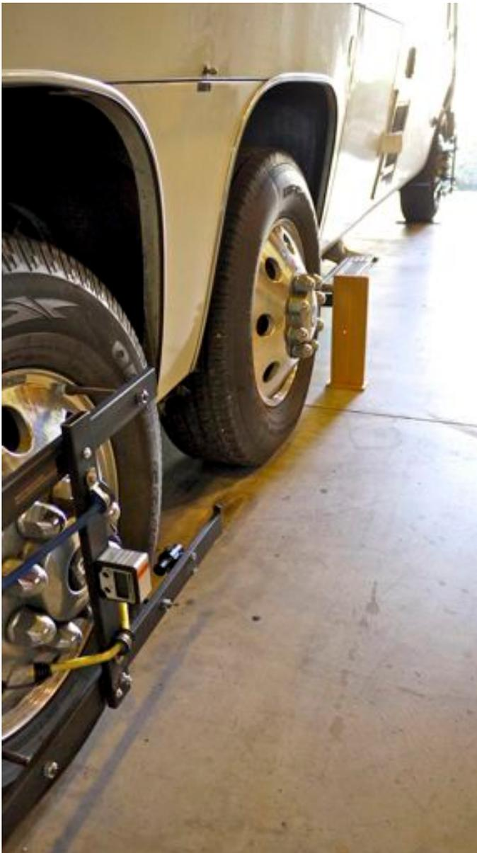
perpendicular to the wheel and zero it. Magnetically attach the angle meter to the vertical upright member and directly read camber. Record that reading.
