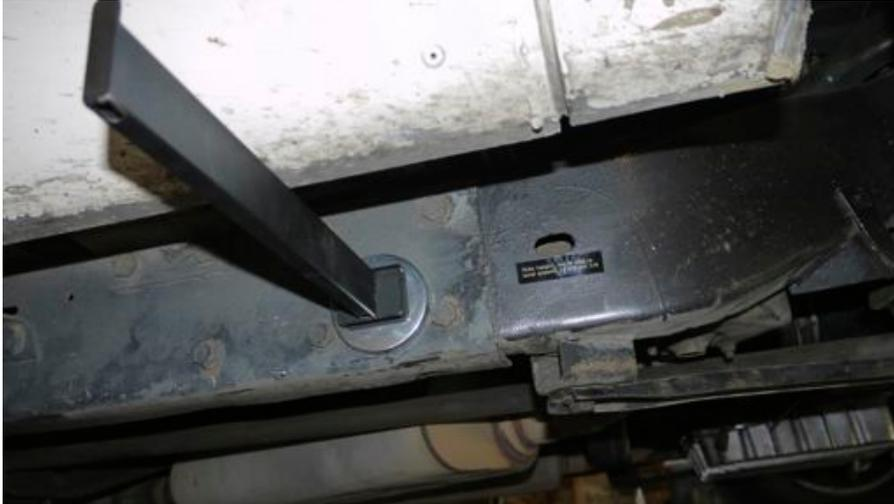
Place the rear arm a bit behind the rear bogie. Be sure the magnets are seated flat against the frame member and not
