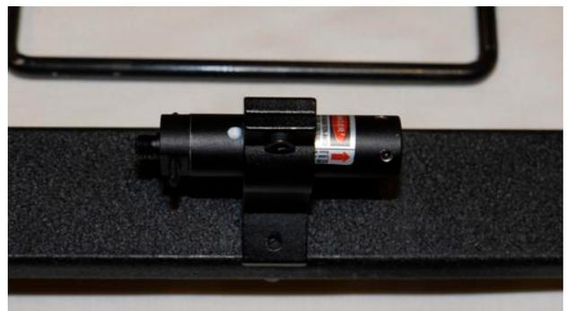
If you damage the laser to the point it no longer functions properly, you can replace it with any 30mm mount gun sight laser. Be sure to calibrate the new one to be parallel with the long arm on the standoff plate.
