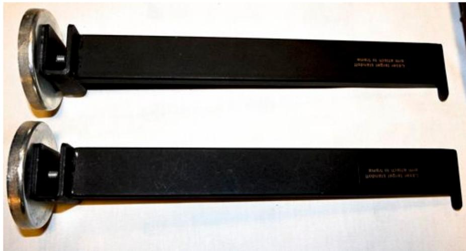
There are two black metal magnetically mounted **frame stand off laser target arms** included with your kit. Follow the instructions to mount these to the frame near the front and rear of the coach. The wooden laser target stands on the ground with one edge aligned to these arms for accurate reading of front and rear wheel parallelism.
