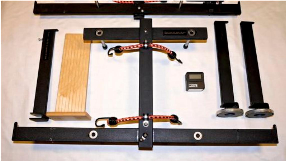
The standoff plates serve as a mounting platform for your Wixey digital angle meter that is coplanar with the rim. The lower arm is fastened at 90 degrees to the upright arm with adhesive and screws. The upper arm is free to pivot to make it easier to mount. The standoff pins are precision machined and come fully calibrated.
