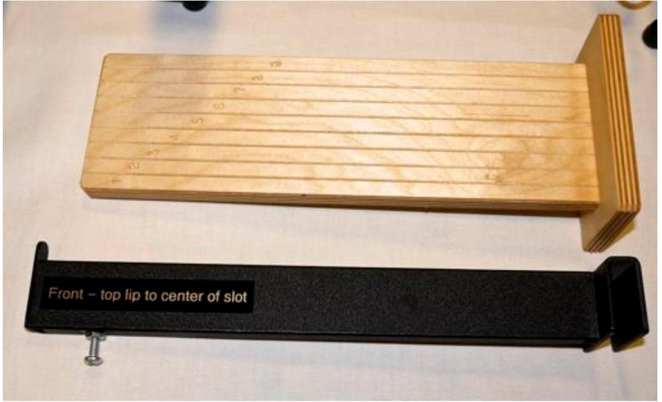
The **wooden laser target** shown above has eight engraved lines 10mm apart on each side. The spaces between these lines are numbered one through nine to make it easy to see where the laser beam hits the target. It is coated with wax to make it easy to wipe off any smudges after use.
