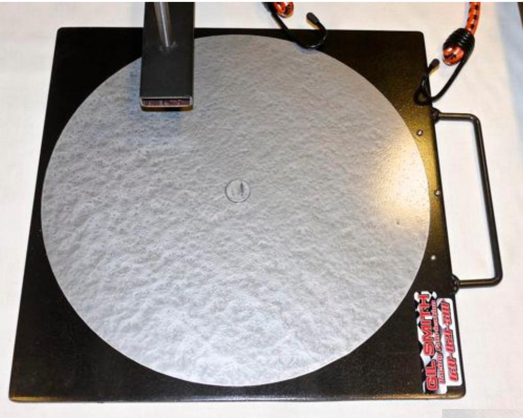
Two **metal turn plates** are included with your kit. They are only 3/8" high so you can drive or push your coach up onto them without lifting your coach or the front wheels off the ground. Each plate features three rivet markers 20 degrees apart. A dry erase marker is included to mark the center point when the wheels have been set pointing parallel with the frame. These will normally be drop shipped directly to you from my supplier to save duplicate shipping cost.
