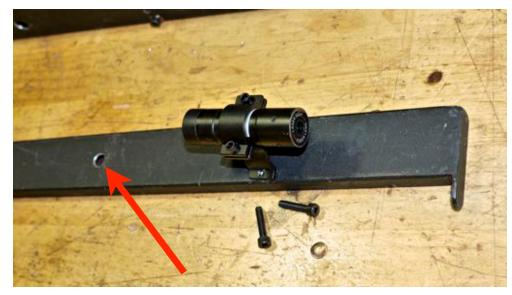
these up for now to allow the laser to rotate in the mount. Use the longer 4mm screws to attach the mount to the long arm with the laser pointing out, off the arm. One laser will be mounted on the right end of one arm and the left end of the other arm. The
