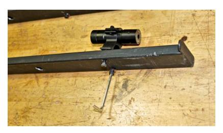
mounting holes are larger than the 4mm screws to allow some small angular adjustment of the mount. Use the 4mm wave washer on the lower attachment screw as shown below. Note the tab on the end of the lower arm. That tab will be pointing up when the arm is assembled onto the rest of the stand off plate components.
