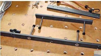
epoxy. Put the vertical member over those two barrel nuts and screw in two SS 10 x 24 screws to hold these two components together. While not critical, it is a good idea to make sure the lower arm and vertical member are at right angles to one another. Use a square to set them, and then tighten the screws snugly.
