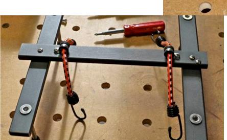
The final step is to screw the bungie cords to the vertical members with SS 10 x 24 screws and the padded clamps. This will keep the bungie cords from getting lost over time.
