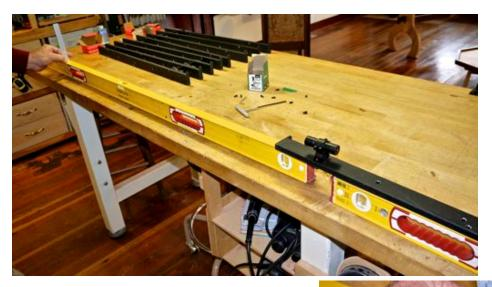
You want those two measurements to be the same. Adjust the height of the laser beam by rotating the laser in the mount. The actual laser itself is set at an angle so rotating the laser will shift the beam up or down as well as left and right. You want the laser to be parallel with the arm and you don't care where it goes side to side. In most
