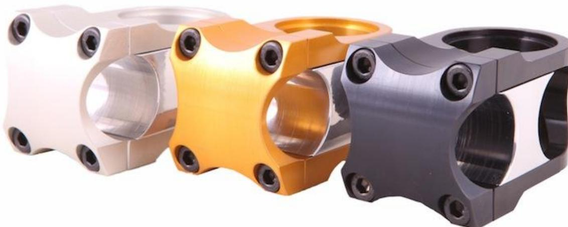
**Stems:** Dedicated to the art of Bike Polo, the S-42 stem is machined from solid block, 7075-T6 alloy and uses an innovative clamping system for easy installation. Also, weighing in at 4.8 oz, this stem is half the weight of a classic BMX stem and a short length (42 mm) for maximum maneuverability and control. Finally, eliminating the back bolt helps riders avoid knee injuries while in the field.
