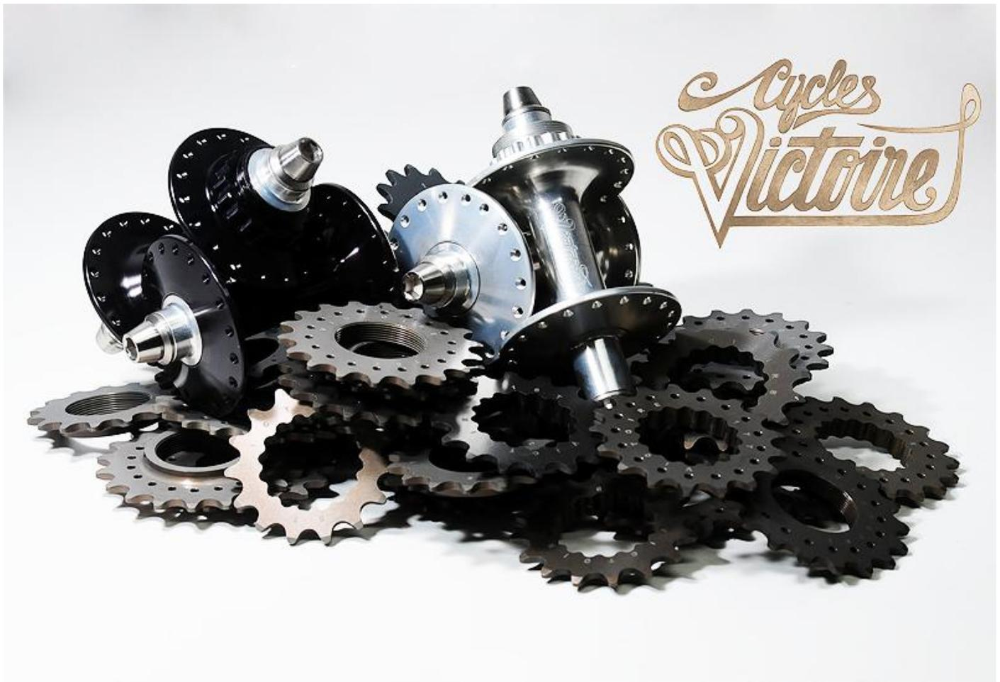
**Cogs:** Designed with a splined interface to eliminate loosened thread on hubs, the interface has 16 splines and no sharp edges to distribute and diffuse the effort on all surfaces. They are available in one tooth increments from 13 to 20 teeth.
