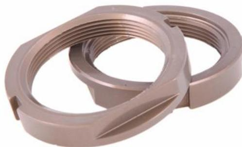
**Lockrings:** An essential part of fixy bikes, the lockring is designed to work with either the Victoire rear hub or any track hub that use the 1.29X24 TPI left thread. Both strong and light, the Victoire lockring is larger than most models available on the market. Made with 7075-T6 alloy, it is 7mm thick, anodized to improve stiffness and can be locked with a lockring wrench or a 36mm wrench.
