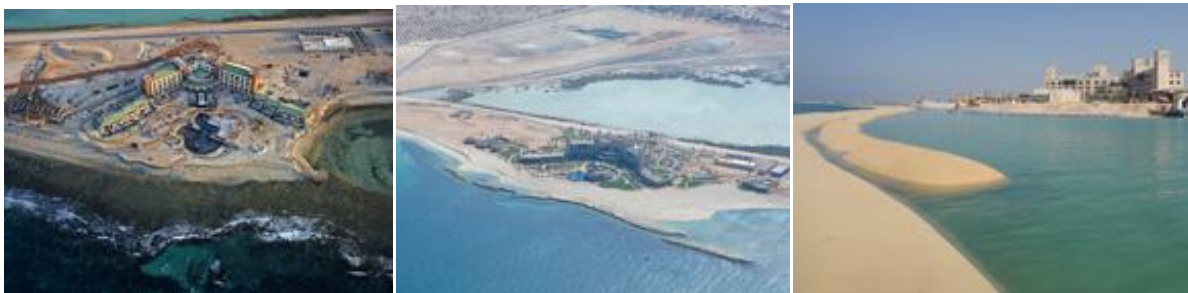
Figure 2 Example of semi submerged reef breakwater constructed of sand filled geotextile containers in the UAE.
