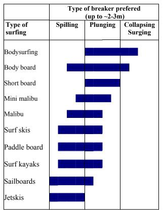
Figure 3 – Type of surfing vs. type of breaker
