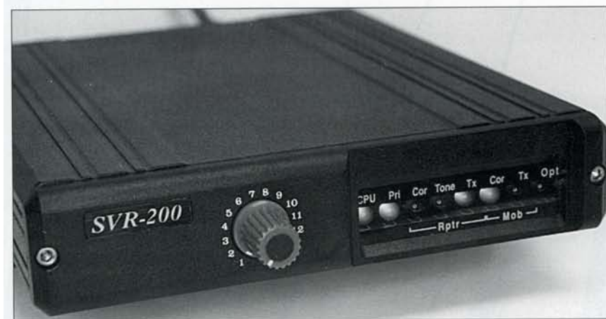
Vehicular repeaters offer a cost-effective means of linking two systems together, in addition to extending handheld range.
