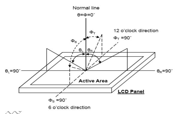
Fig. 8-1 Definition of viewing angle
