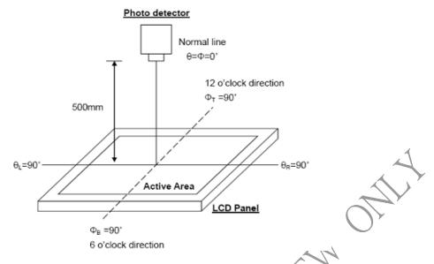
Fig. 8-2 Optical measurement system setup
