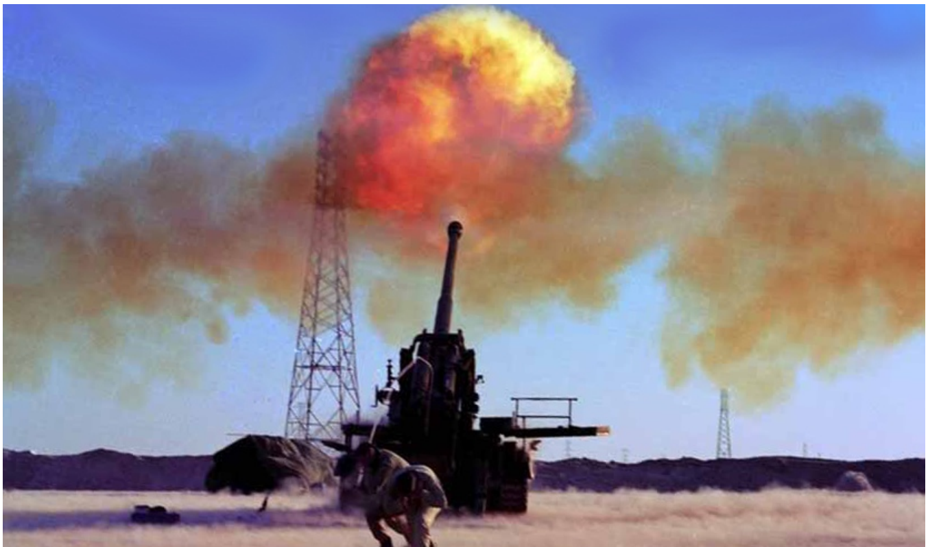
A restored photograph of an Iranian M-1978 firing. Note the crew platform swung out to the right side and large blast. ( www.sajed.ir )
