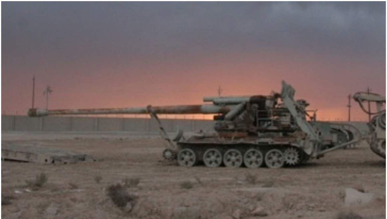
Another view of what appears to be a 180 mm variant of the M-1978 self-propelled gun at al-Anbar University in Ramadi. (U.S. Marine Corps Photo by Lance Cpl. Albert F. Hunt)
