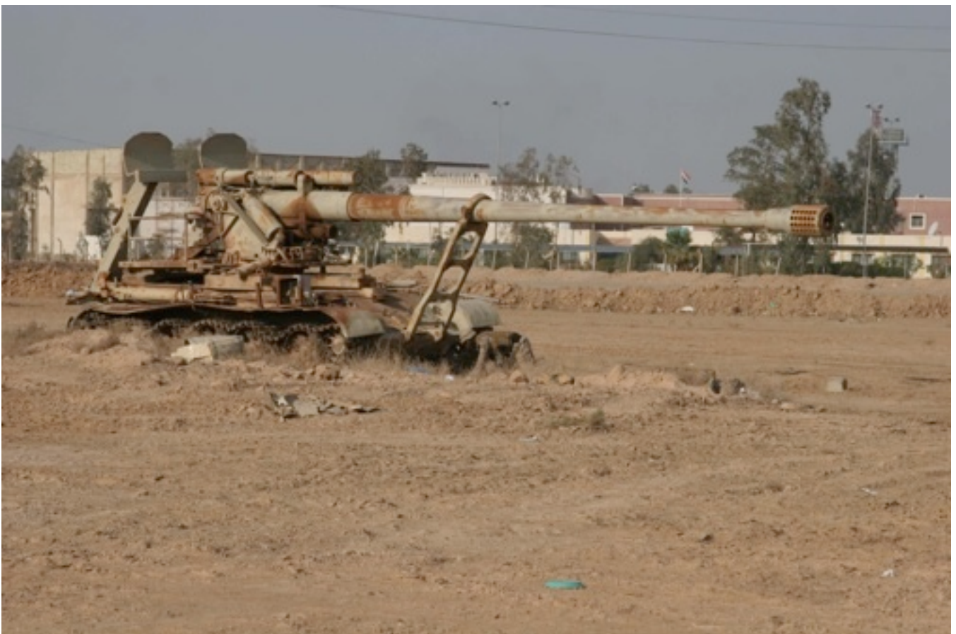
A U.S. Marine Corps image taken in Iraq on November 29, 2008 of what appears to be a 180 mm variant of the M-1978 self-propelled gun. The Marines were working to clear Iraqi tanks from Al Anbar University in Ramadi. When compared to the M-1978 note the barrel shape and the "pepper pot" muzzle brake. (U.S. Marine Corps Photo by Lance Cpl. Albert F. Hunt)
