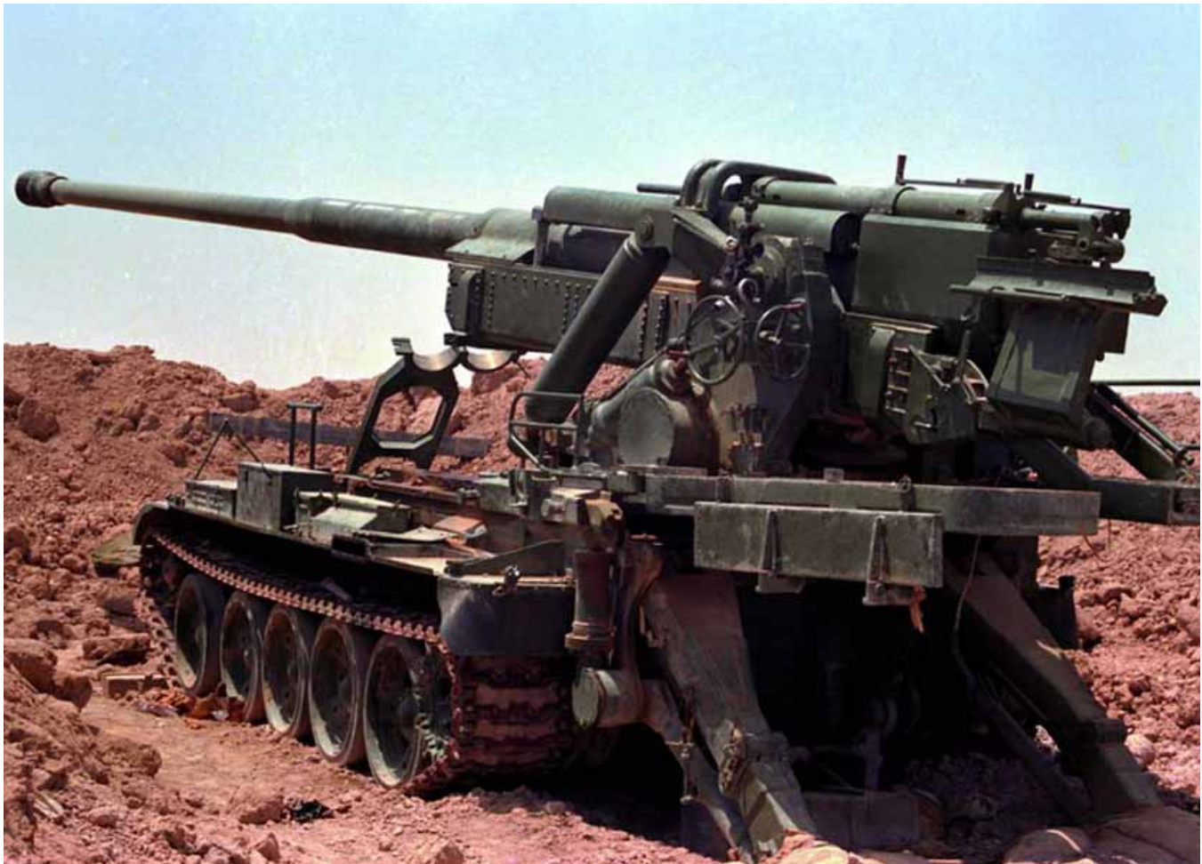
A M-1978 170 mm self-propelled gun in Iranian service deployed within a revetted firing position. (www.sajed.ir)
