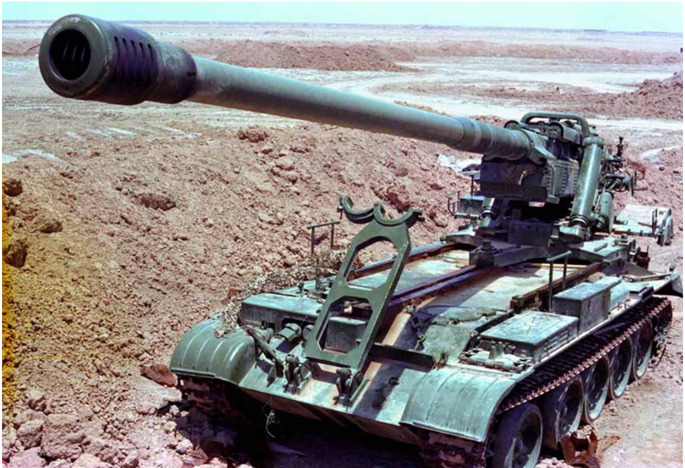
A DPRK produced M-1978 170 mm self-propelled gun in service with the Iranian Army. ( www.sajed.ir )
